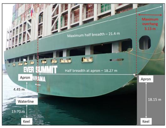
Figure 15. The *Ever Summit's* maximum overhang at the stern at the time of the occurrence (Source: TSB)
