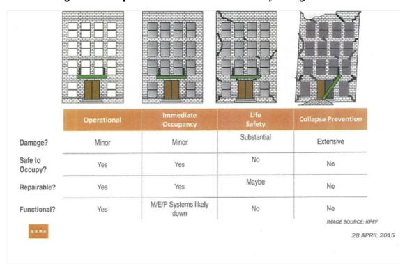
OPS would likely suffer significant damage during a major seismic event, and seismic infrastructure improvements would be required to bring the building up to an "Immediate Occupancy" or "Operational" standard.
