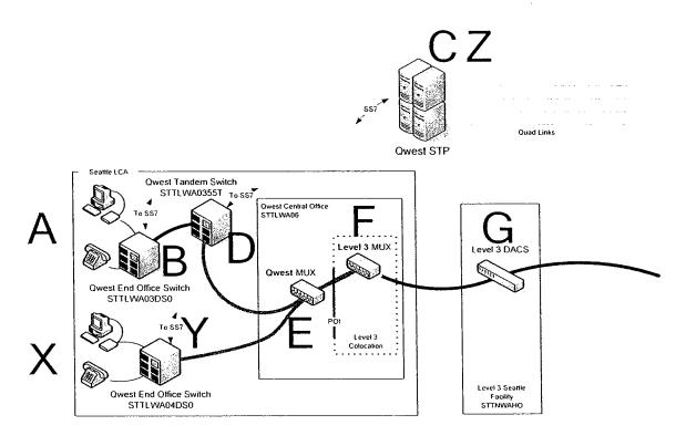
In Seattle the Level 3 network connects with Qwest either through trunks at a tandem switch to get to an end office such as the relationship between STTLWA0355T (Tandem) and STTLWA03DS0 or the Level 3 network connects directly to the Qwest End office such as STTLWA04DS0. Both types of connects come back to Level 3 collocation site at STTLWA06
