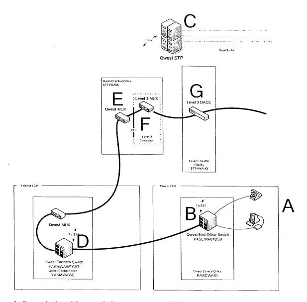
In Pasco the Level 3 network does not connect with Qwest in the Local Calling Area creating a VNXX arrangement through Yakima. VNXX traffic represents less than 1% of traffic exchanged between Level 3 and Qwest.
