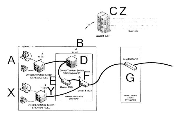
In Spokane the Level 3 network connects with Qwest either through trunks at a tandem switch to get to an end office such as the relationship between SPKNWA01C9T (Tandem) and OTHEWA01DS0 or the Level 3 network connects directly to the Qwest End office such as SPKNWAFADS0. Both type of connections come back to the Level 3 network end point established at SPKNWA01 which services as a POI. Level 3 has established this network end point by leasing separate DS3 networks from both ELI and Qwest
