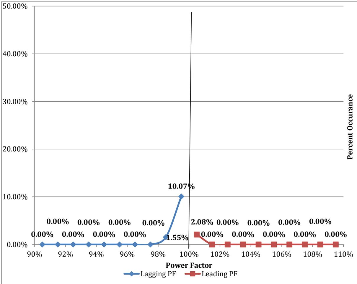
**Figure 25. Proposed Percent Occurrence of Power Factor with net 600 kVAR Installed**
