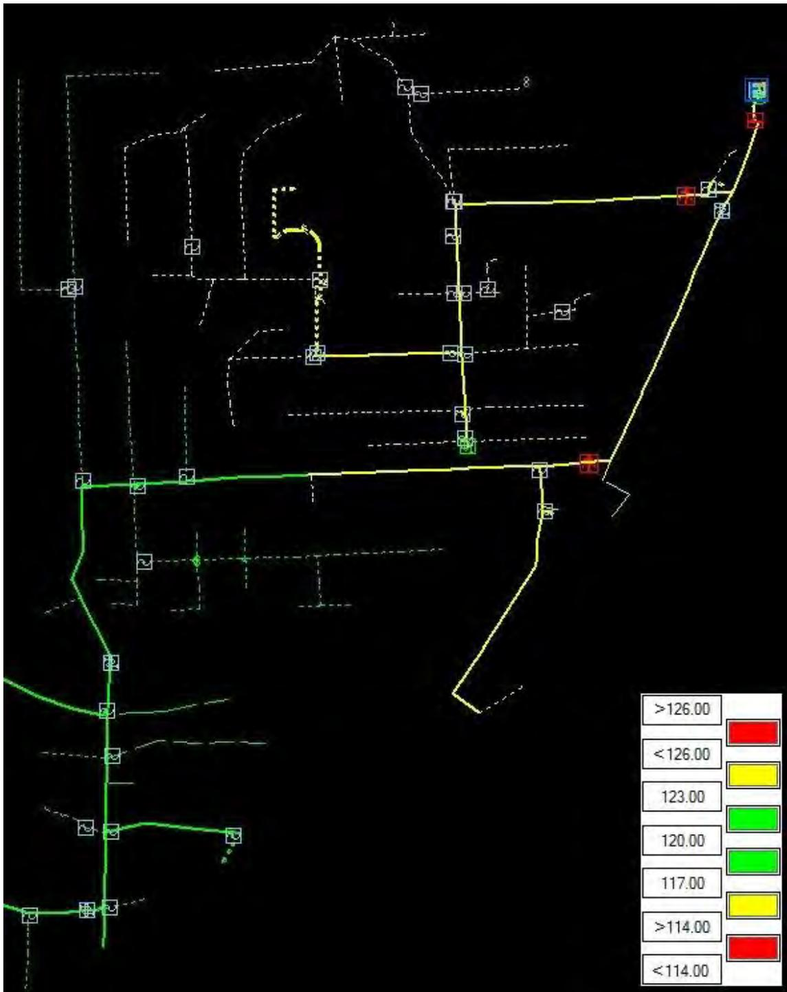
Figure 14. High Voltage Levels Modeled at Peak Loading
