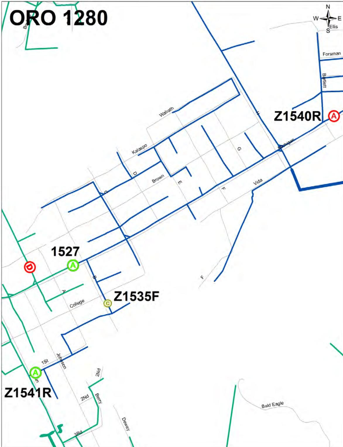
Figure 11. ORO 1280 Proposed Automation Device Locations
