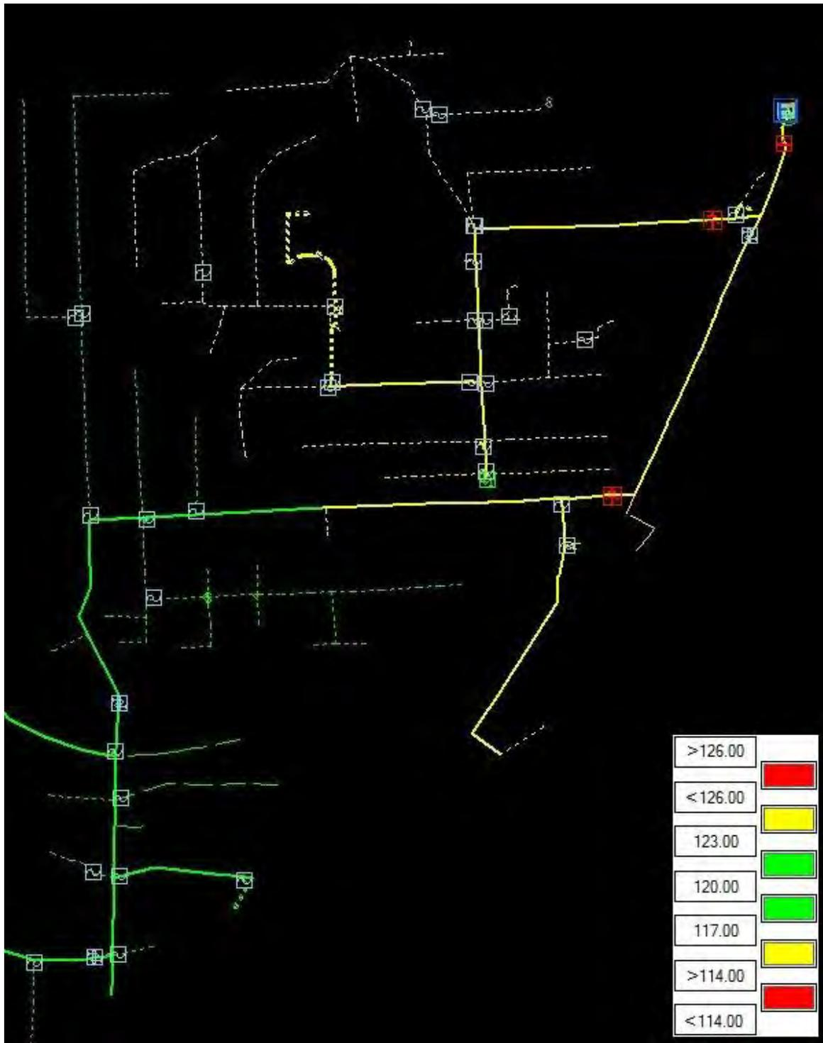
Figure 12. High Voltage Levels Modeled at Peak Loading
