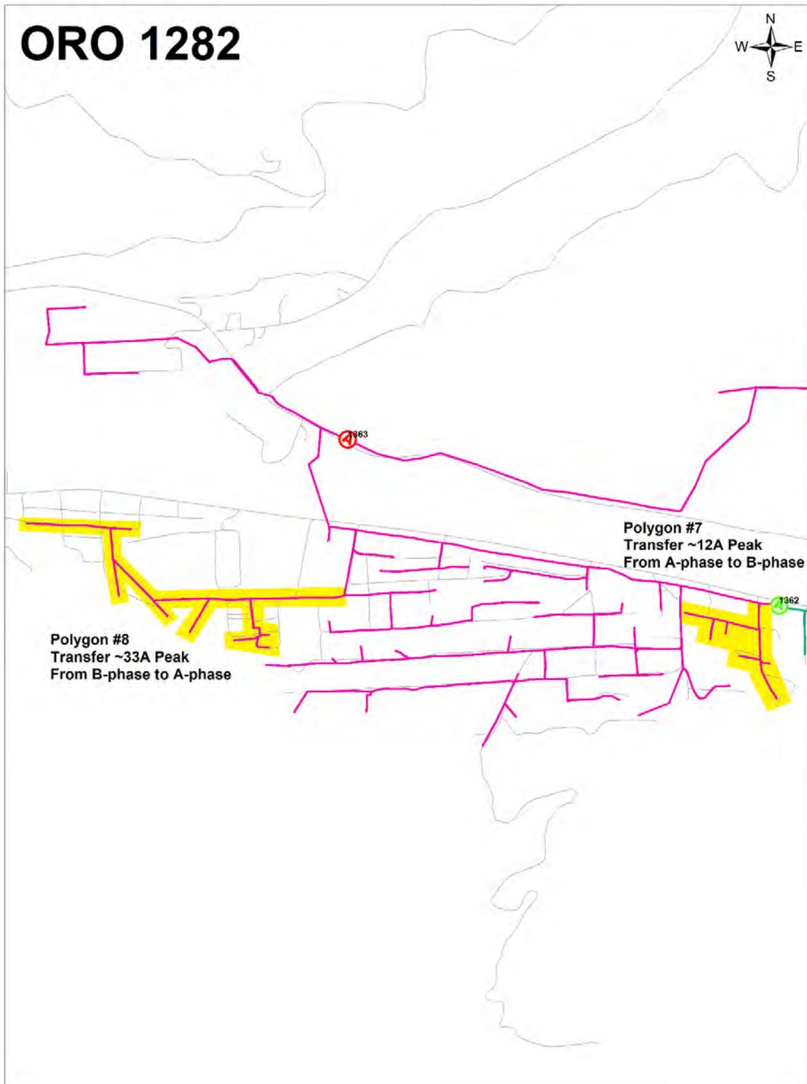
**Figure 13. ORO 1282 Feeder Load Balancing Phase Change Recommendations**
