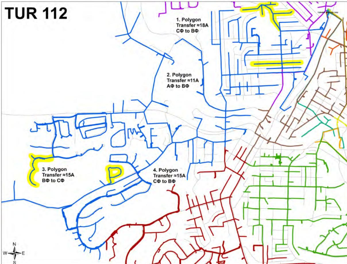
**Figure 3. Feeder Balancing – Recommended Phase Changes**
