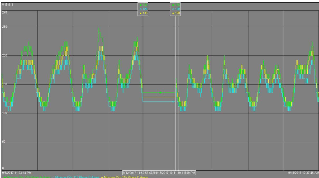
**Figure 7. M15 514 Abnormal Feeder Configuration Reflecting Additional Loading**
