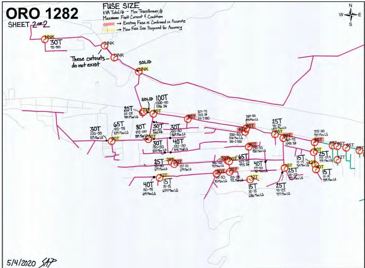
Figure 32. Fuse Size & Coordination Recommendations, Sheet 2 of 2
