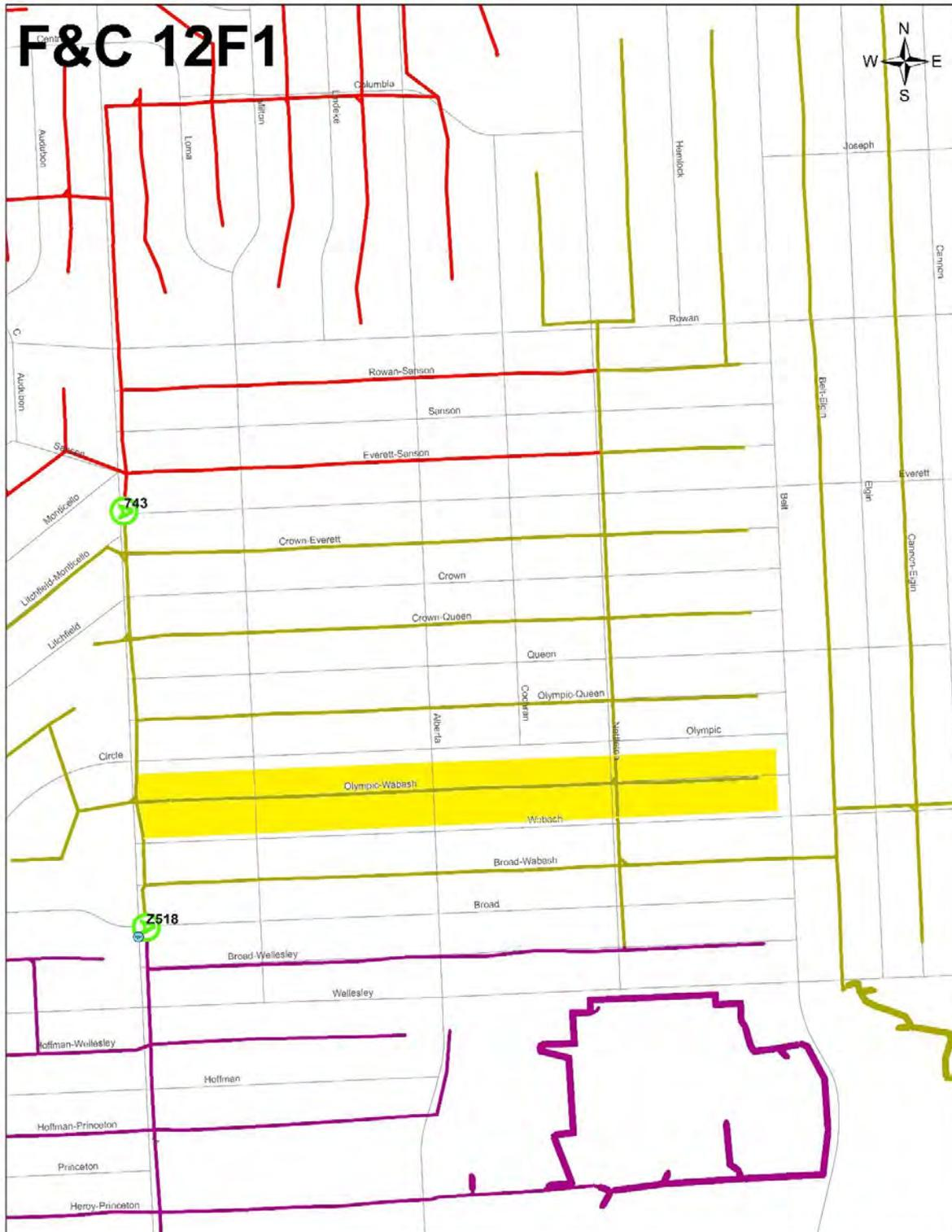
**Figure 6. Polygon 5 Primary Lateral Recondutor to 4 ACSR**
