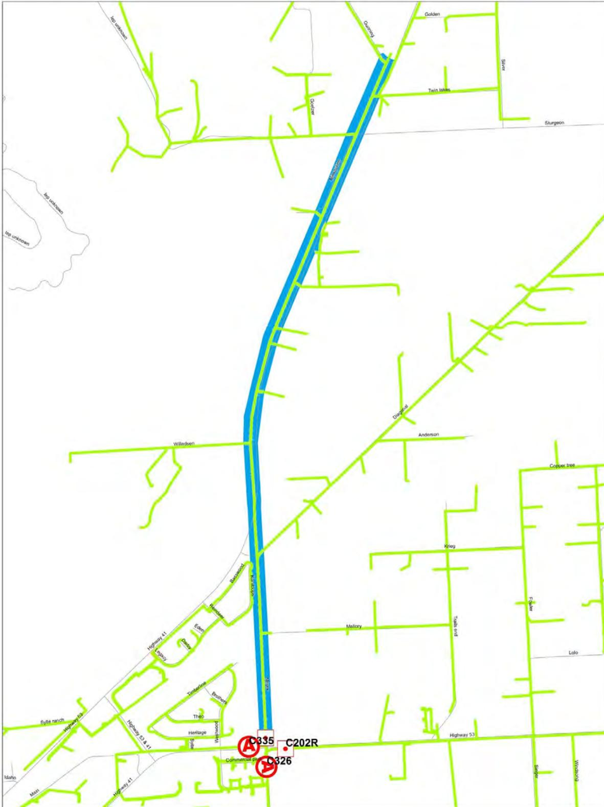
Figure 4. Polygons 6 and 9 Primary Reconductor to 2/0 ACSR
