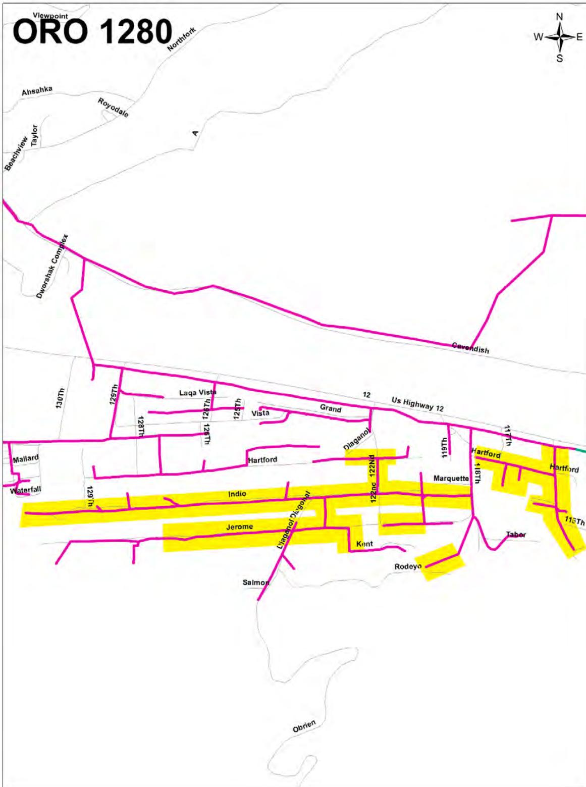
Figure 19. 6CU Primary Laterals Requiring Reconductor
