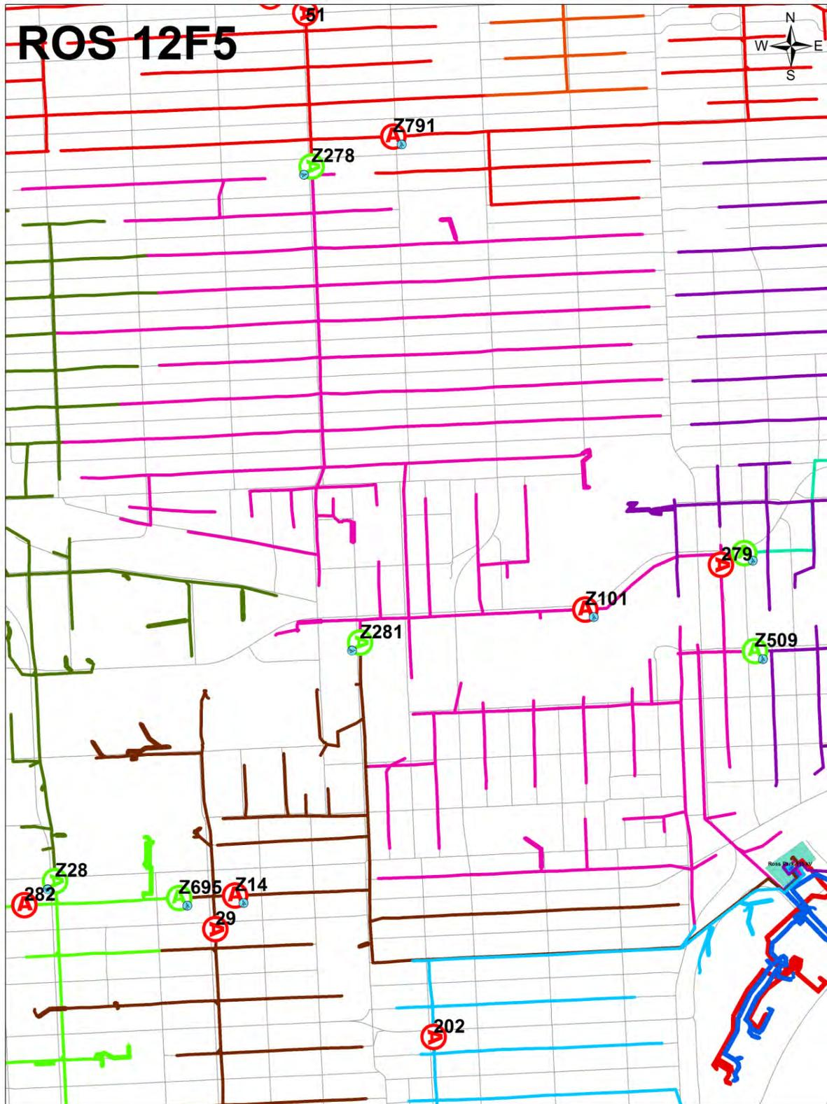
Figure 12. ROS 12F5 Distribution Feeder Tie Devices
