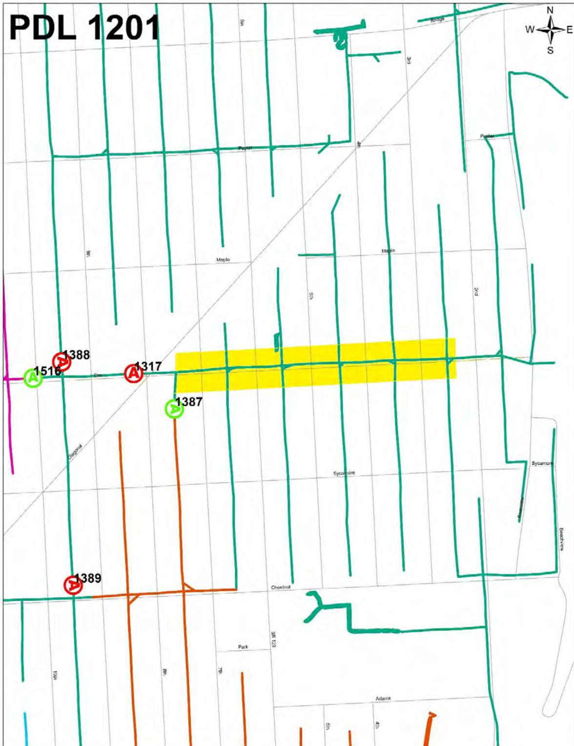
Figure 4. Polygon 5 Three-Phase Lateral Reconductor to 336 AAC
