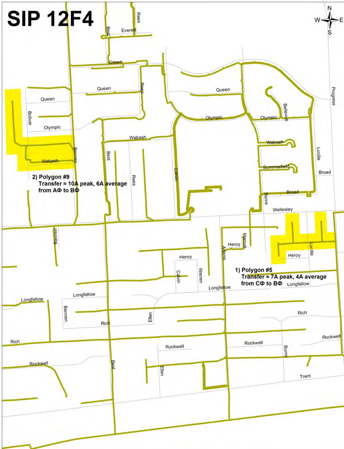
Figure 10. SIP 12F4 Load Balancing on Polygons 5 and 9
