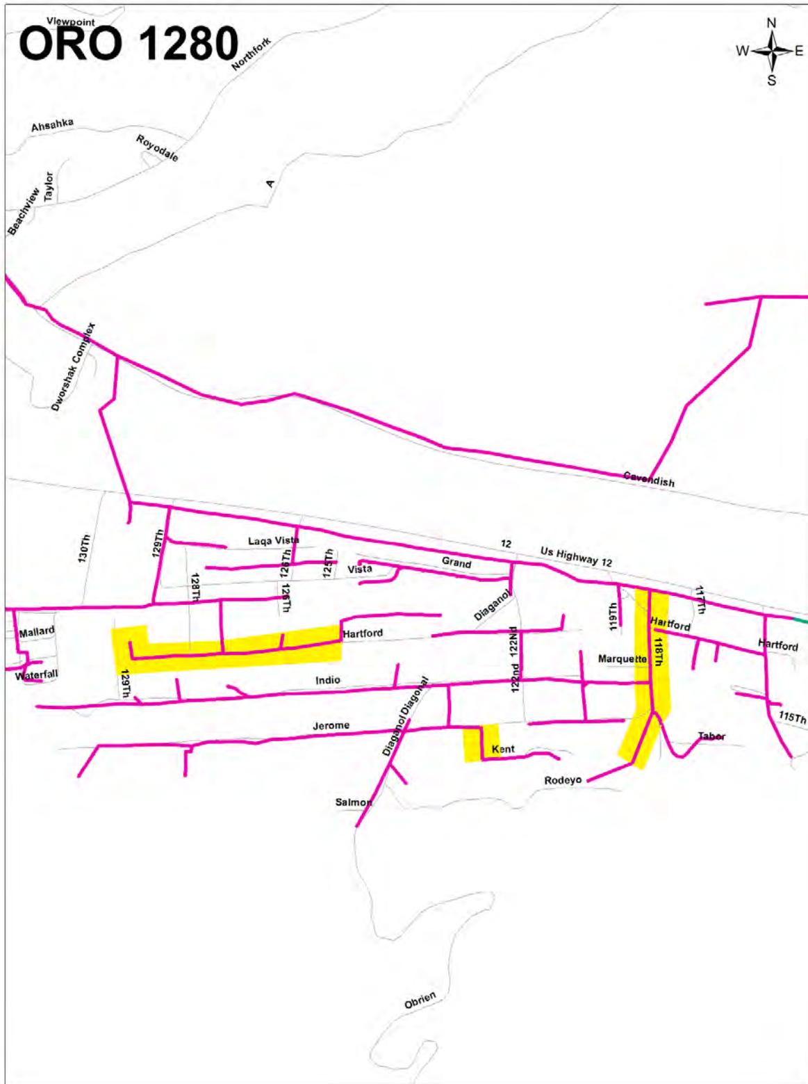
Figure 17. 6A Primary Laterals Requiring Reconductor
