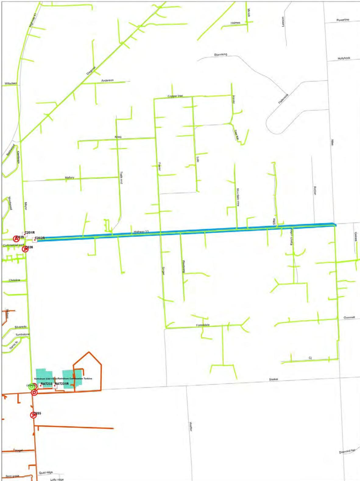
Figure 3. Polygons 2 and 4 Primary Reconductor to 2/0 ACSR
