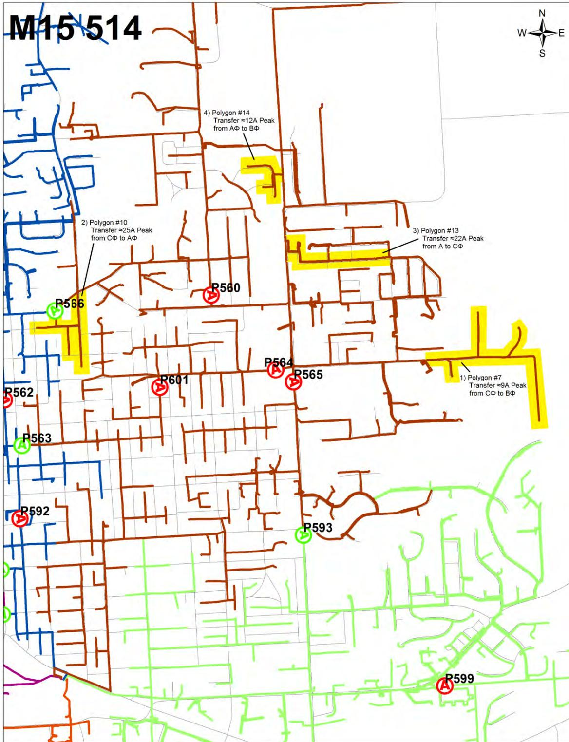
Figure 8. M15 514 Feeder Balancing – Recommended Load Transfers
