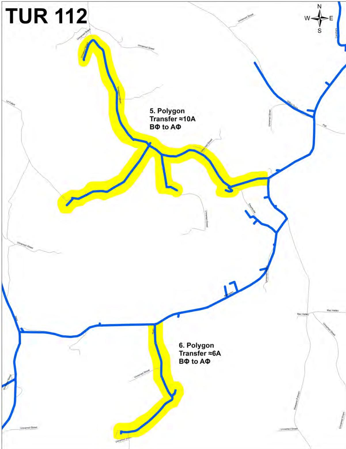
Figure 4. Feeder Balancing – Recommended Phase Changes
