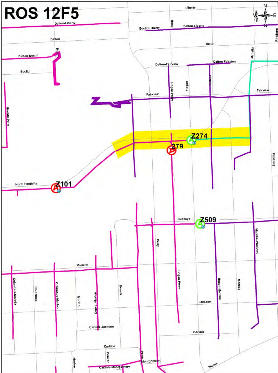
Figure 11. ROS 12F5 Primary Trunk Reconductor to 556AAC
