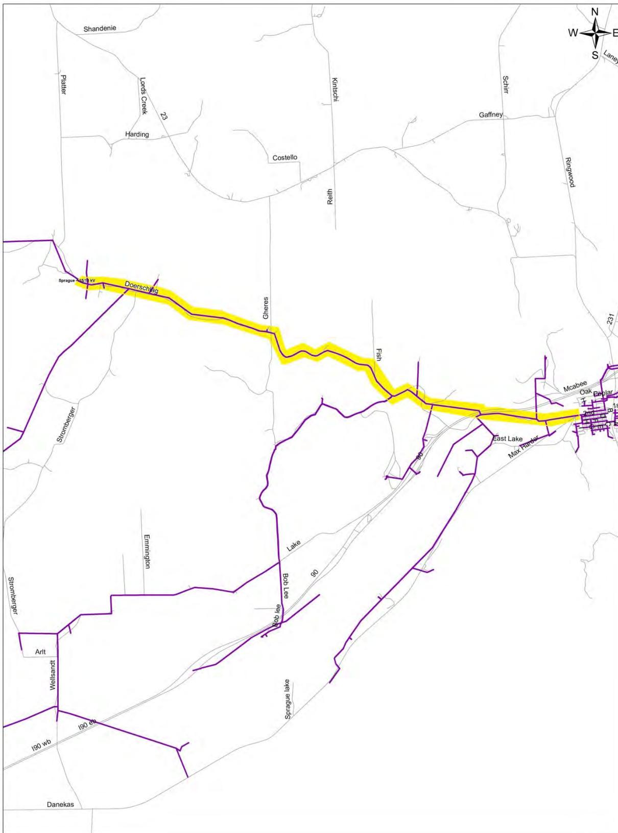
**Figure 4. Polygons 1, 2, 3, 4, 5, 6 and 7 Reconductor to 2/0 ACSR**
