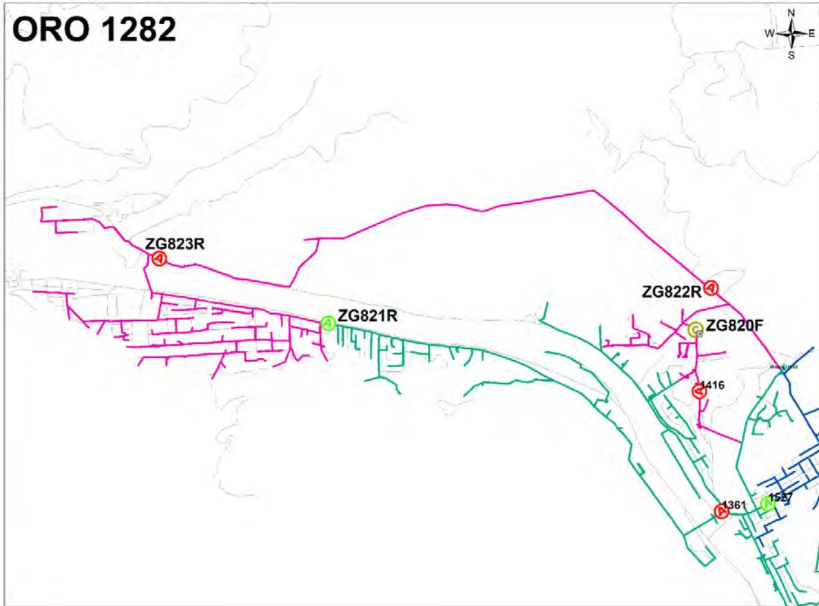
Figure 36. Distribution Line Automation Device Locations on ORO 1282
