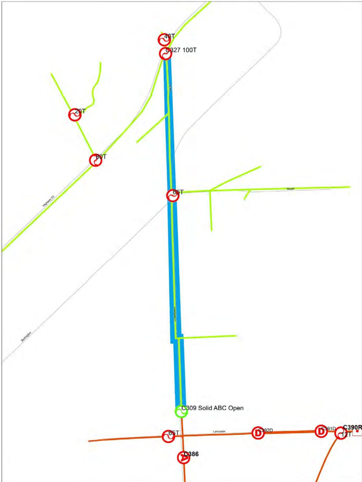
Figure 5. Polygon 21 Primary Reconductor to 2/0 ACSR
