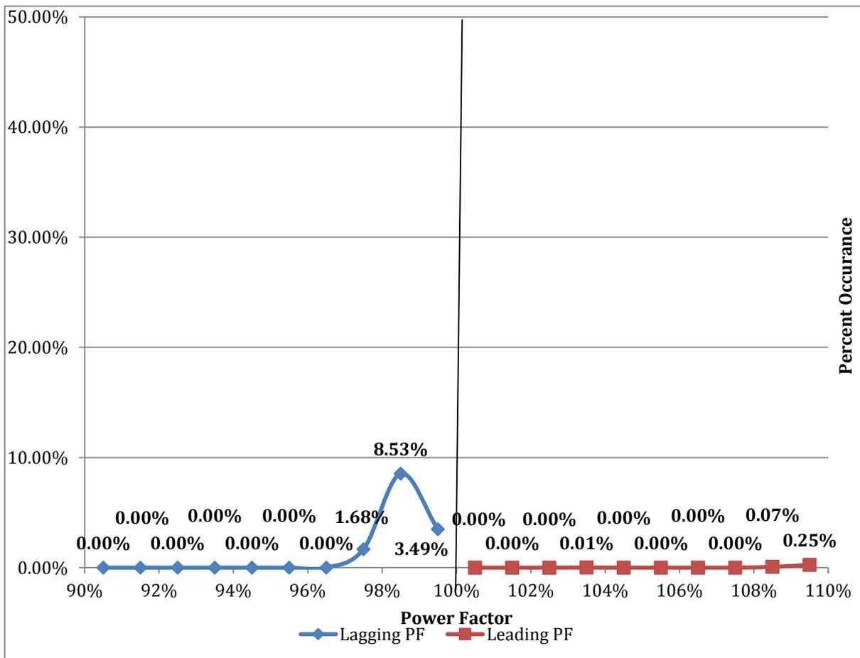
**Figure 24. Proposed Percent Occurance of Power Factor with net 300 kVAR Installed**
