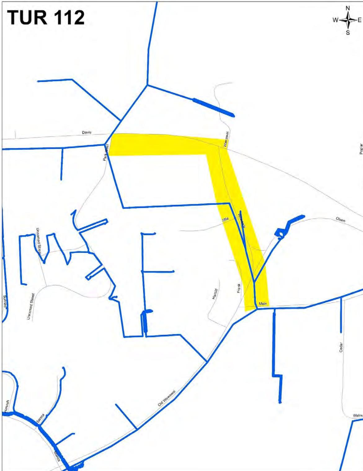
Figure 7. Polygon 4 Feeder Trunk Reconductor to 2/0 ACSR
