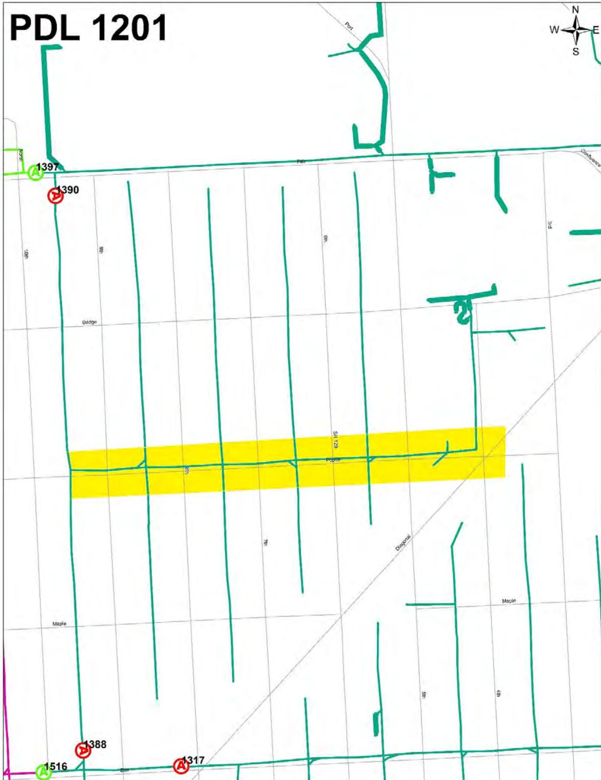
Figure 3. Polygon 6 Three-Phase Lateral Reconductor to 336 AAC
