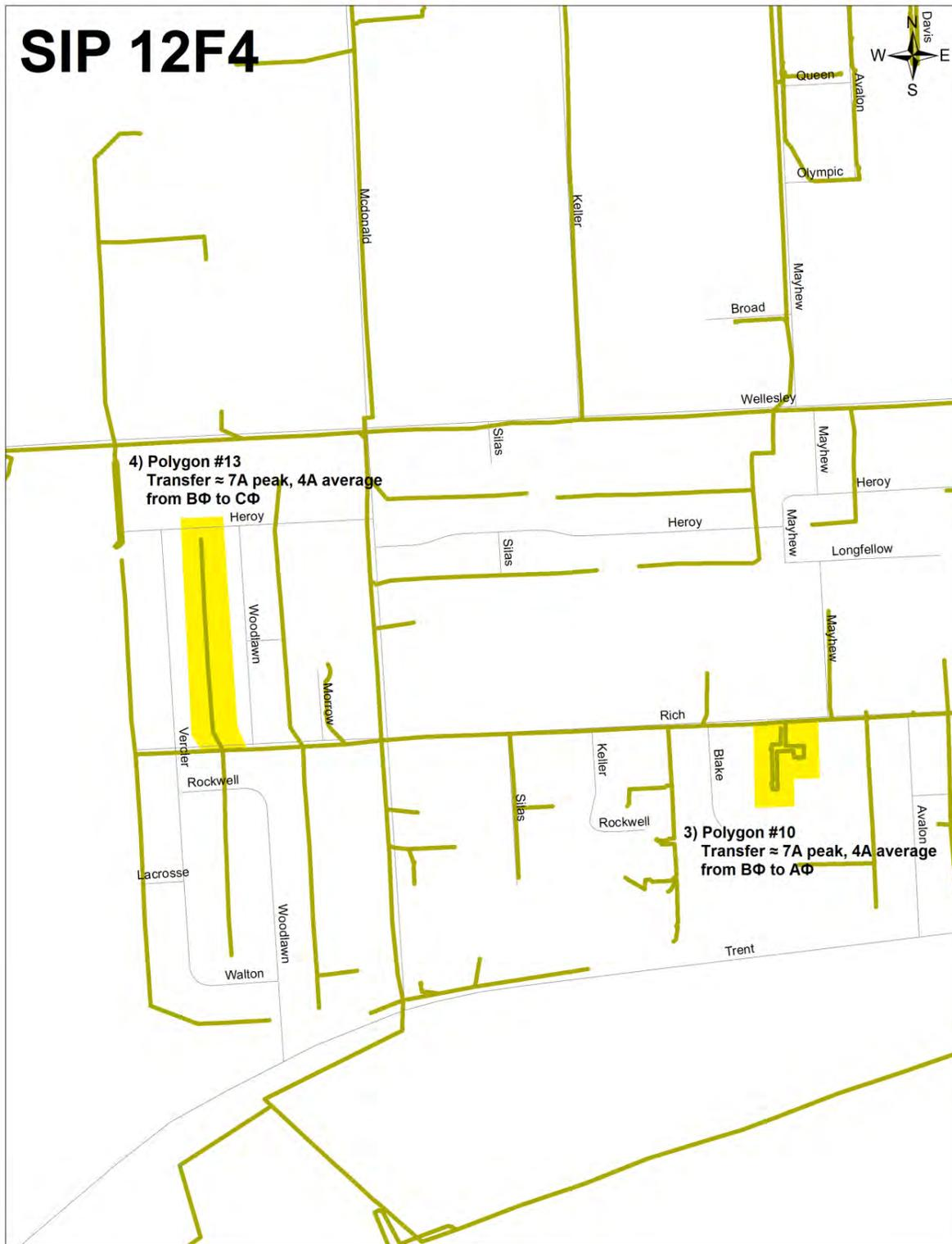
Figure 11. SIP 12F4 Load Balancing on Polygons 10 and 13
