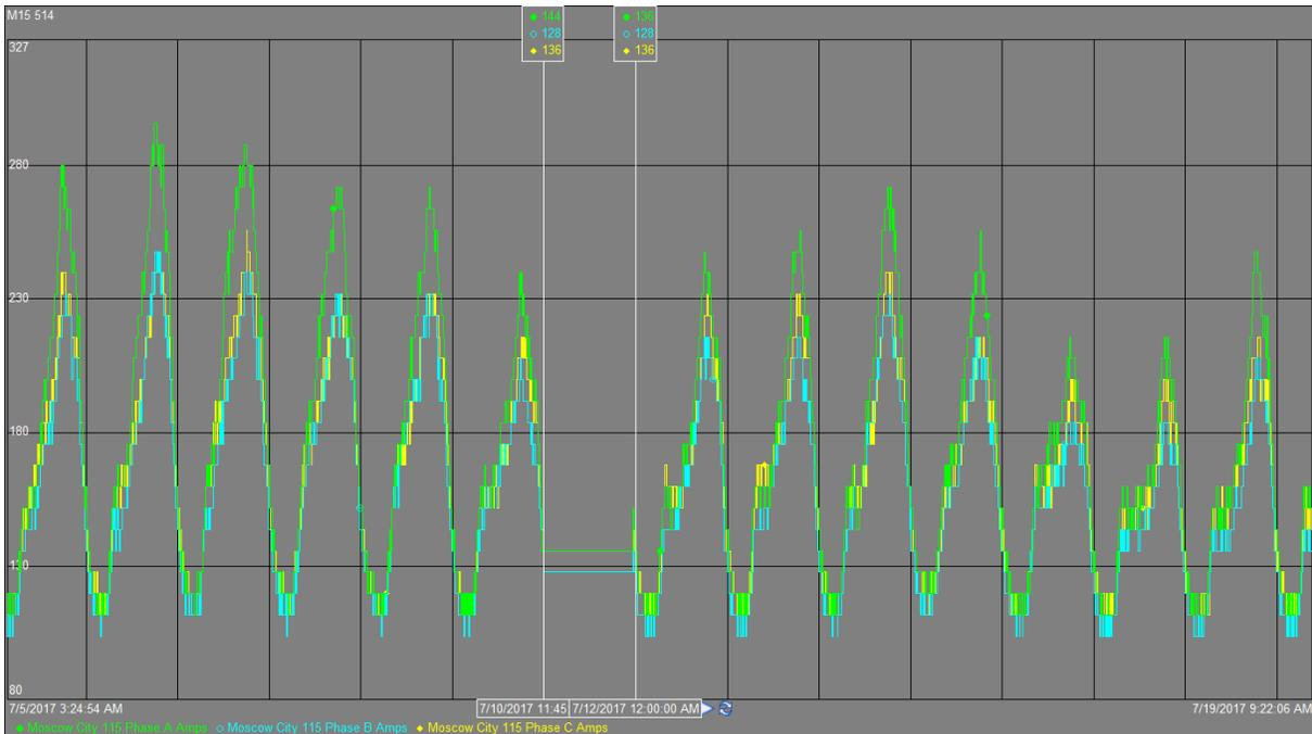
**Figure 6. M15 514 Abnormal Feeder Configuration Reflecting Additional Loading**
