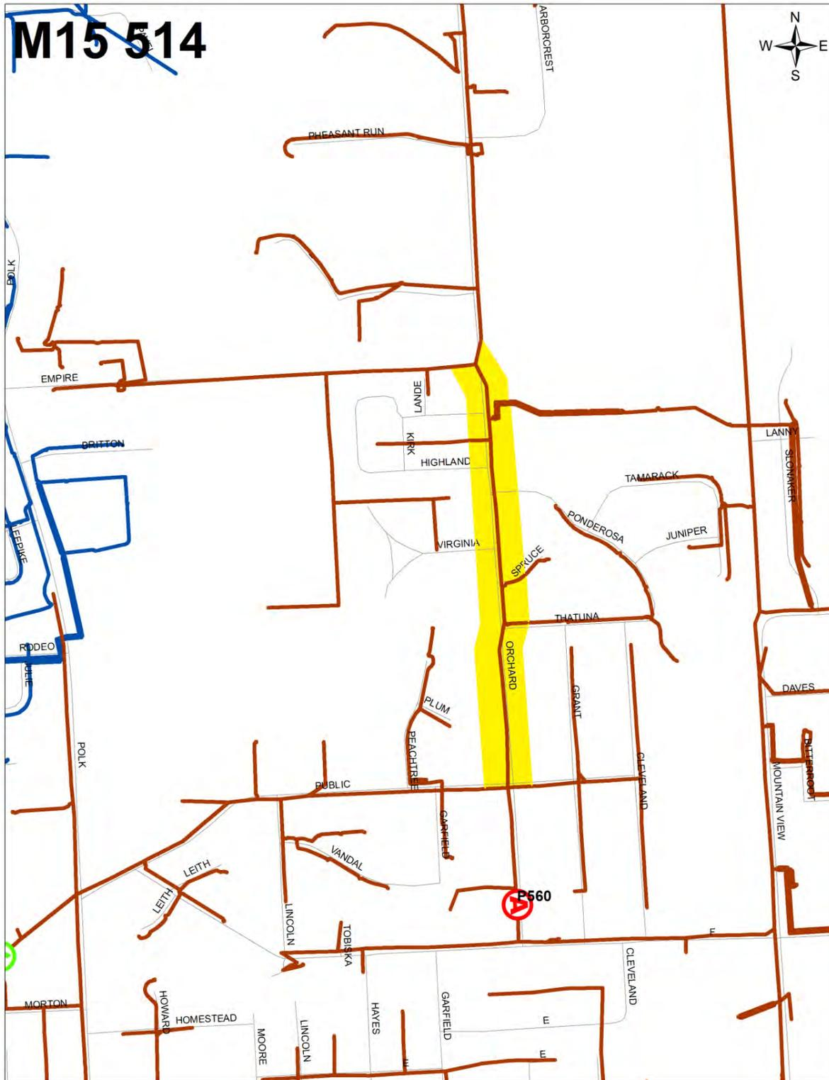
Figure 12. M15 514 Primary Laterals Reconductor in Polygons 9 & 11
