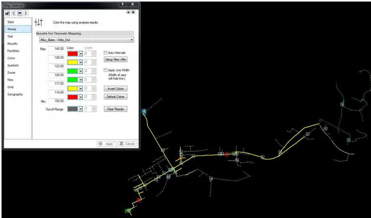
Figure 6. Service Voltage Levels at Peak Load Conditions
