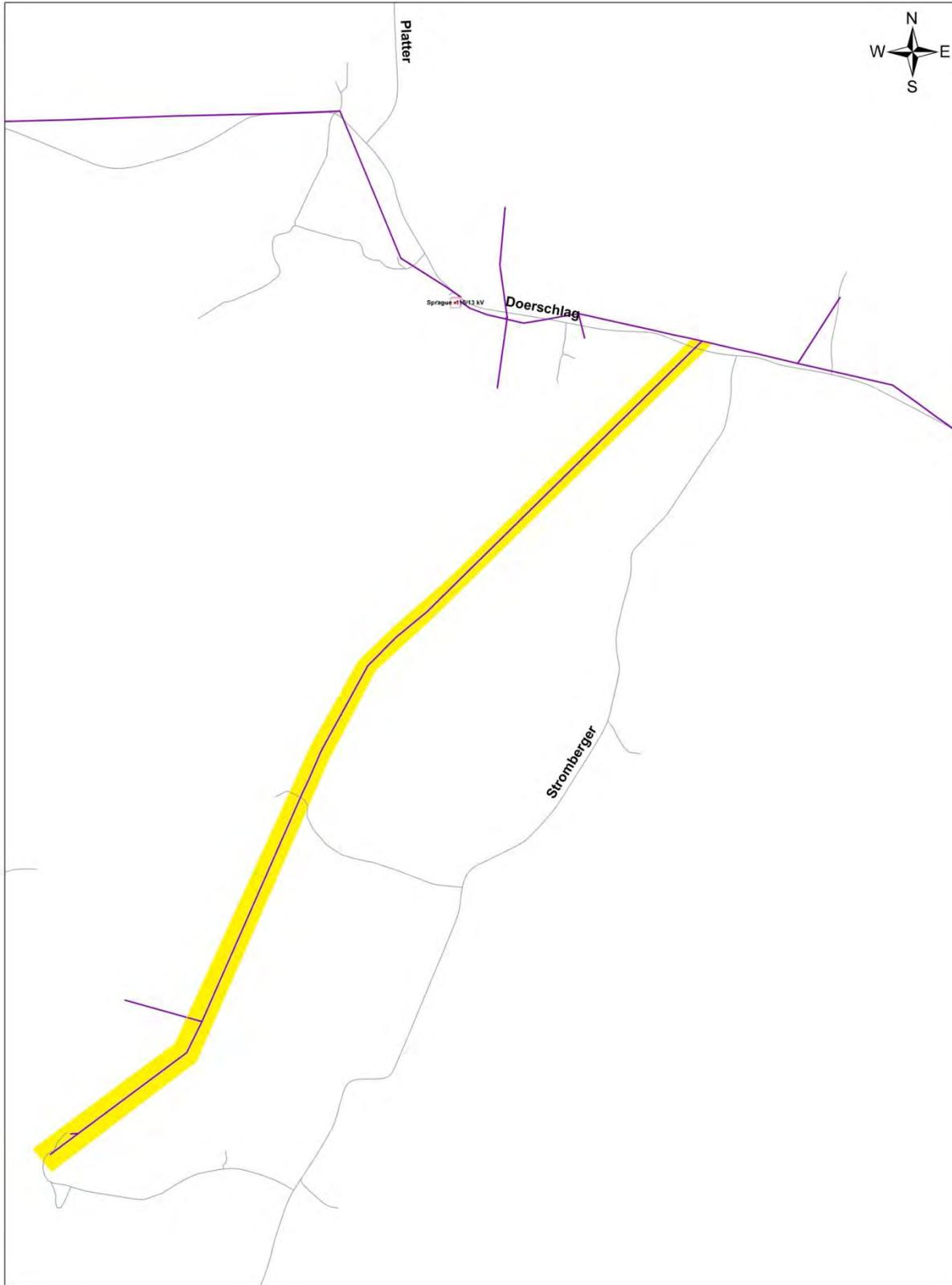
Figure 5. Polygon 27 Lateral Reconfiguration/URD Conversion along Stromberger
