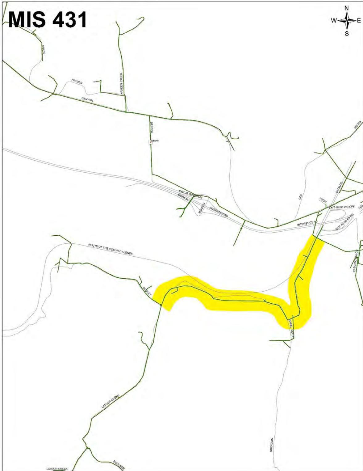
Figure 8. Polygon 6 Add 4 ACSR B-phase to Latour Creek Road Lateral
