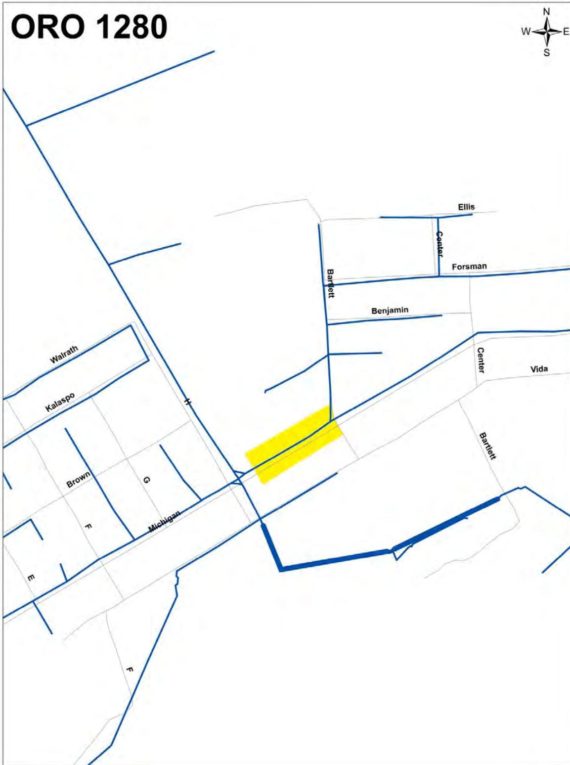
**Figure 4. Polygon 5 Feeder Trunk Reconductor to 2/0 ACSR**
