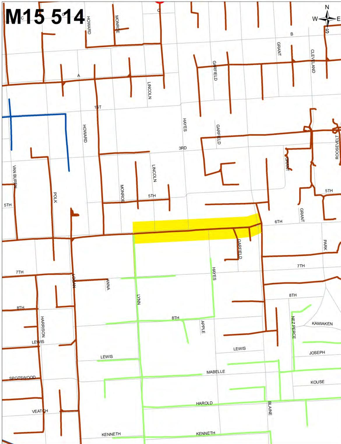
Figure 11. M15 514 Primary Lateral Reconductor in Polygon 2 on E. 6<sup>th</sup> Street
