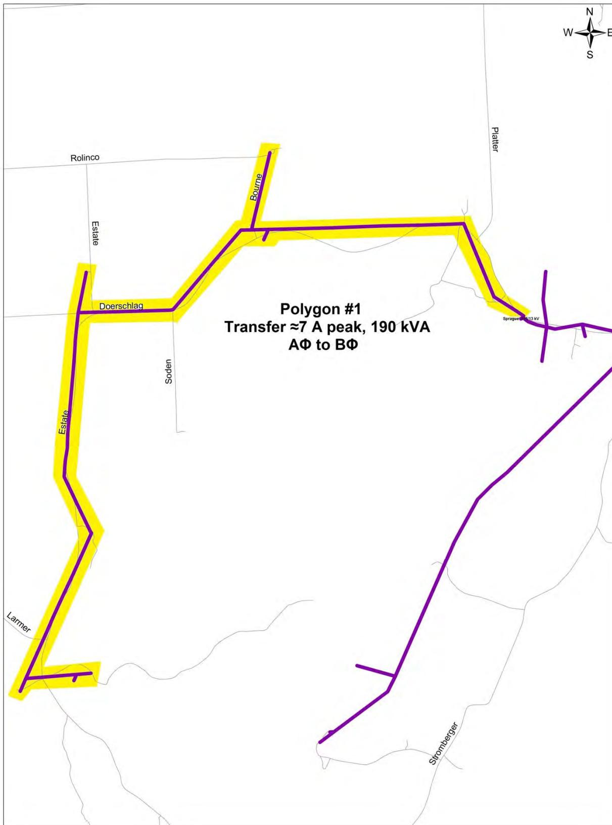
**Figure 2. Feeder Balancing – Recommended Phase Changes**
