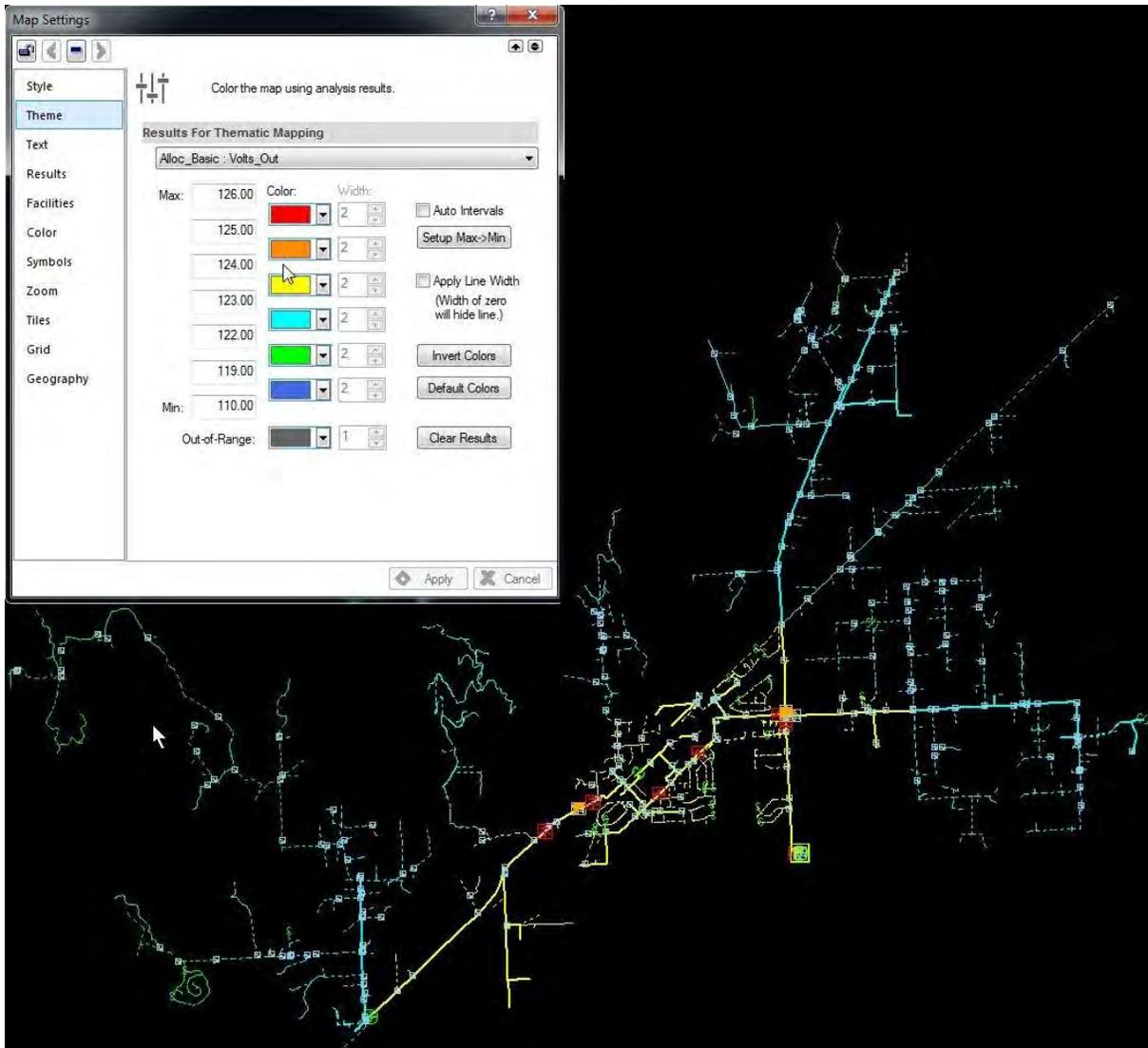
Figure 10. Service Voltage Levels at Median Load Conditions
