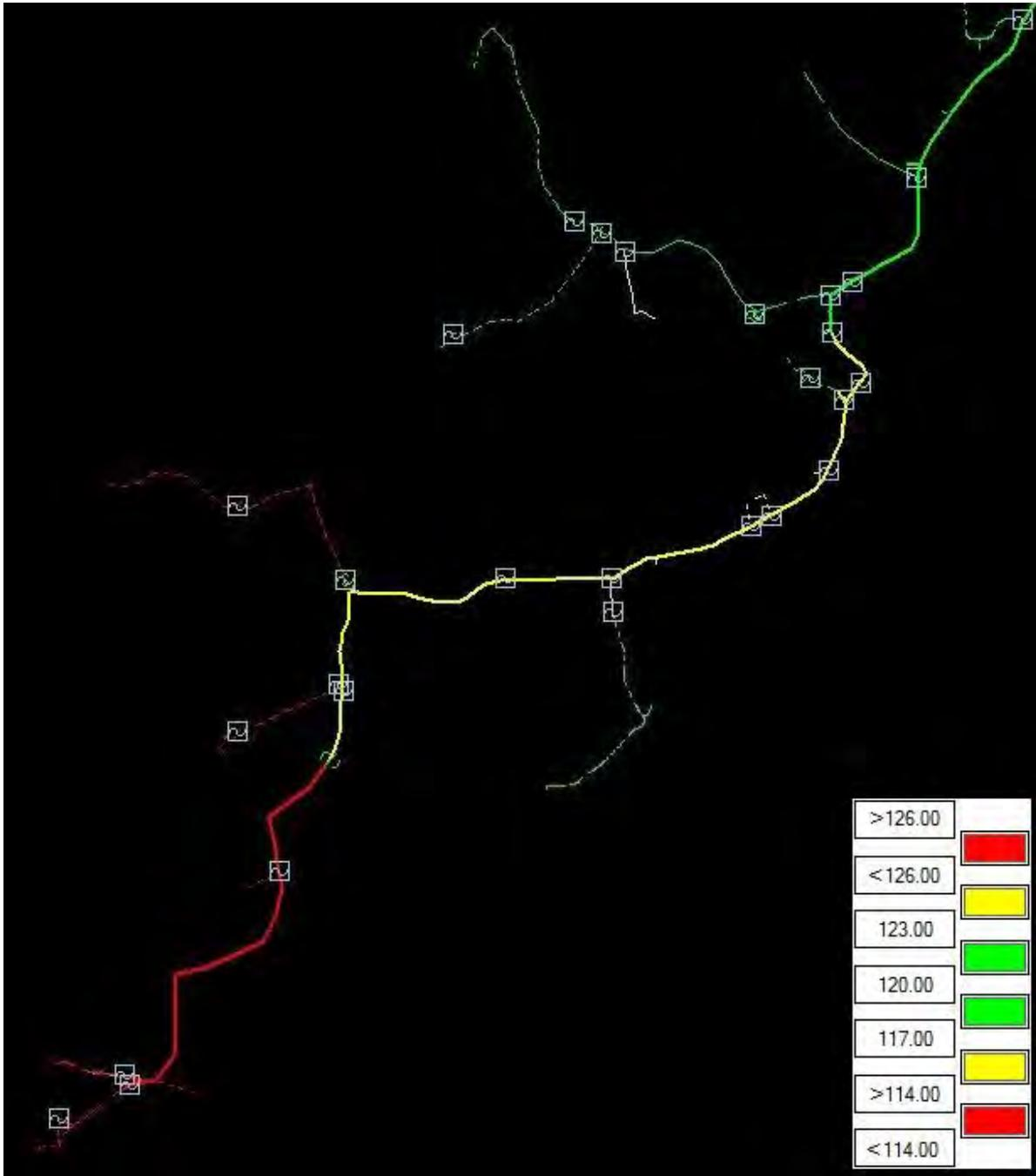
Figure 13. Low Voltage Levels Modeled at Peak Loading
