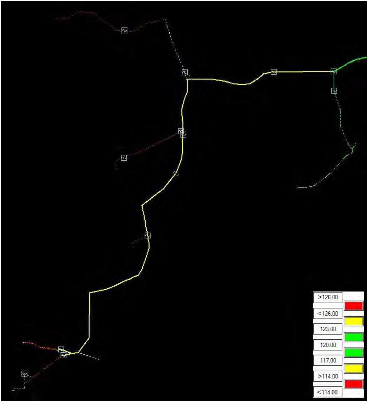
Figure 15. Low Voltage Levels Modeled at Peak Loading
