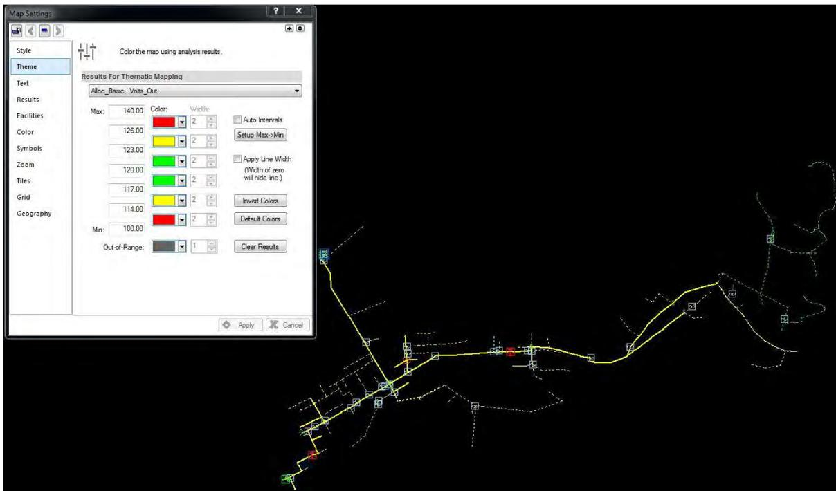
Figure 7. Service Voltage Levels at Median Load Conditions
