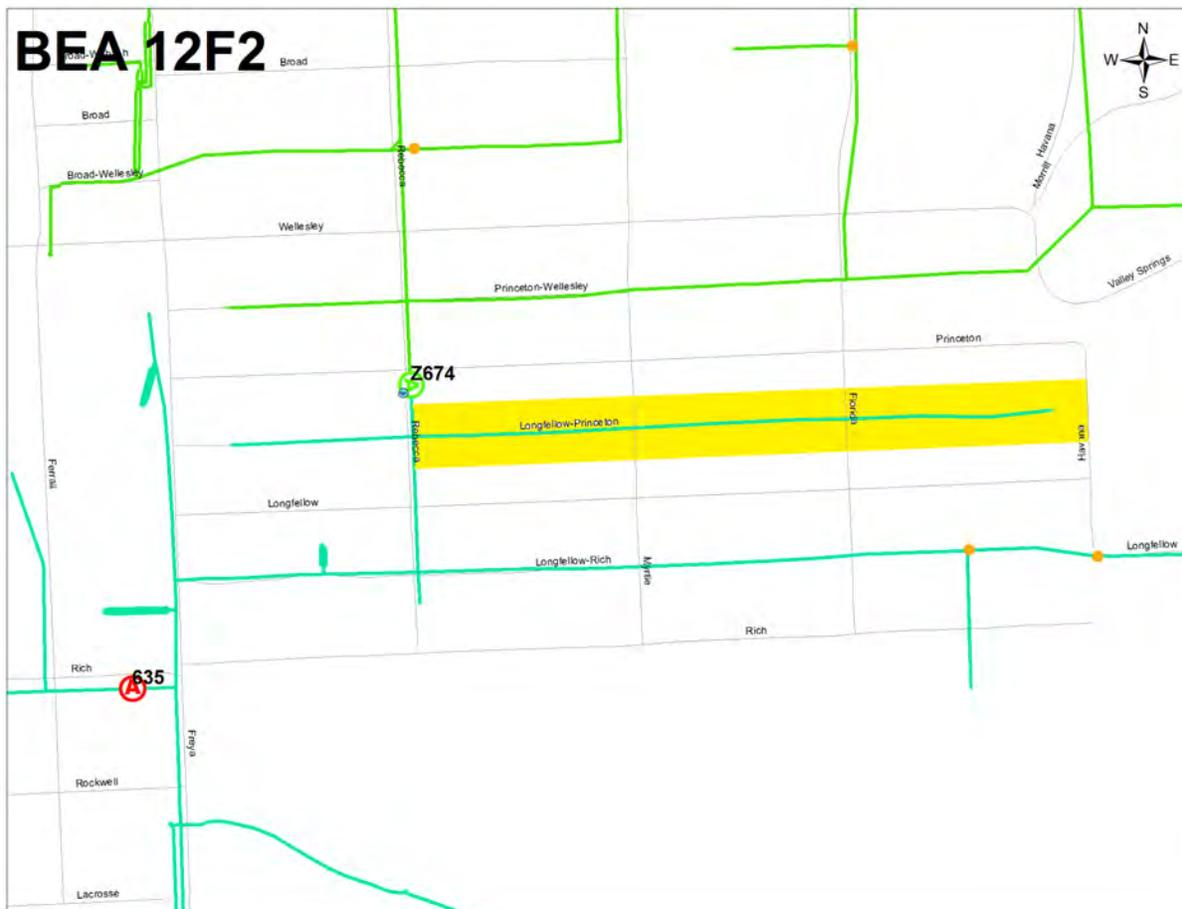
**Figure 12. BEA 12F2 Feeder Balancing – Recommended Phase Change**
