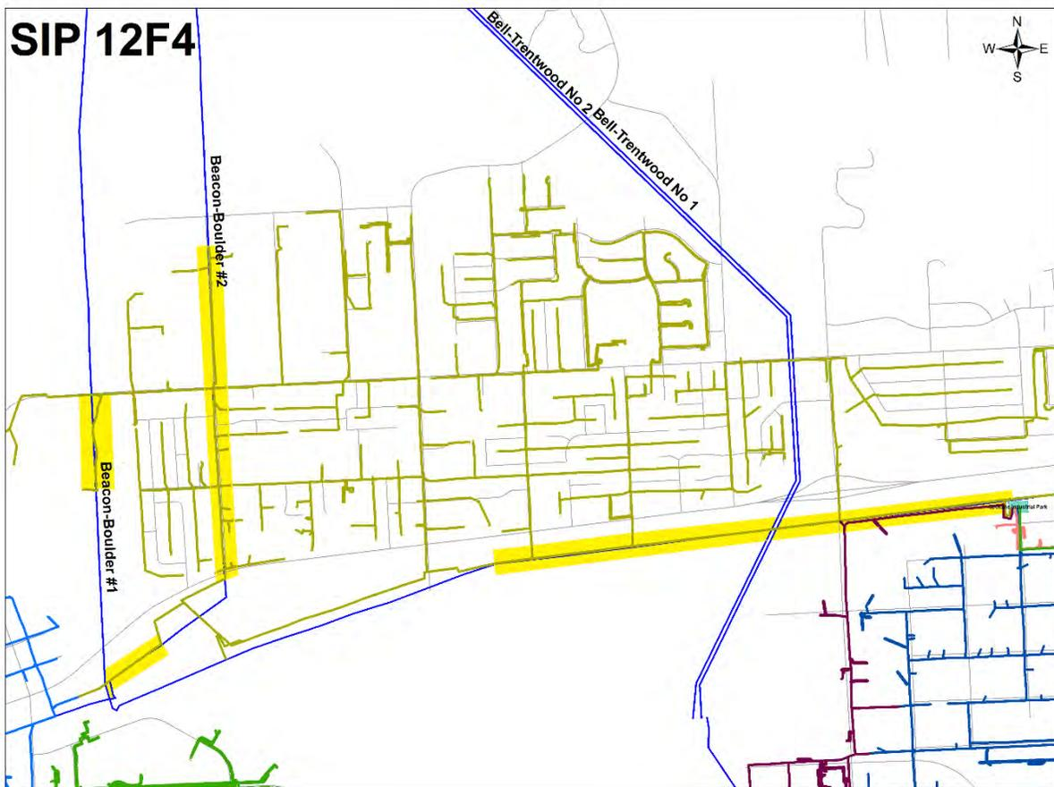
Figure 12. Underbuilt Distribution Primary on Transmission Lines
