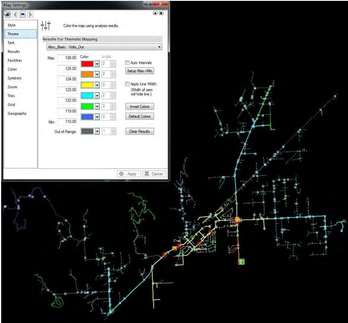
Figure 9. Service Voltage Levels at Peak Load Conditions
