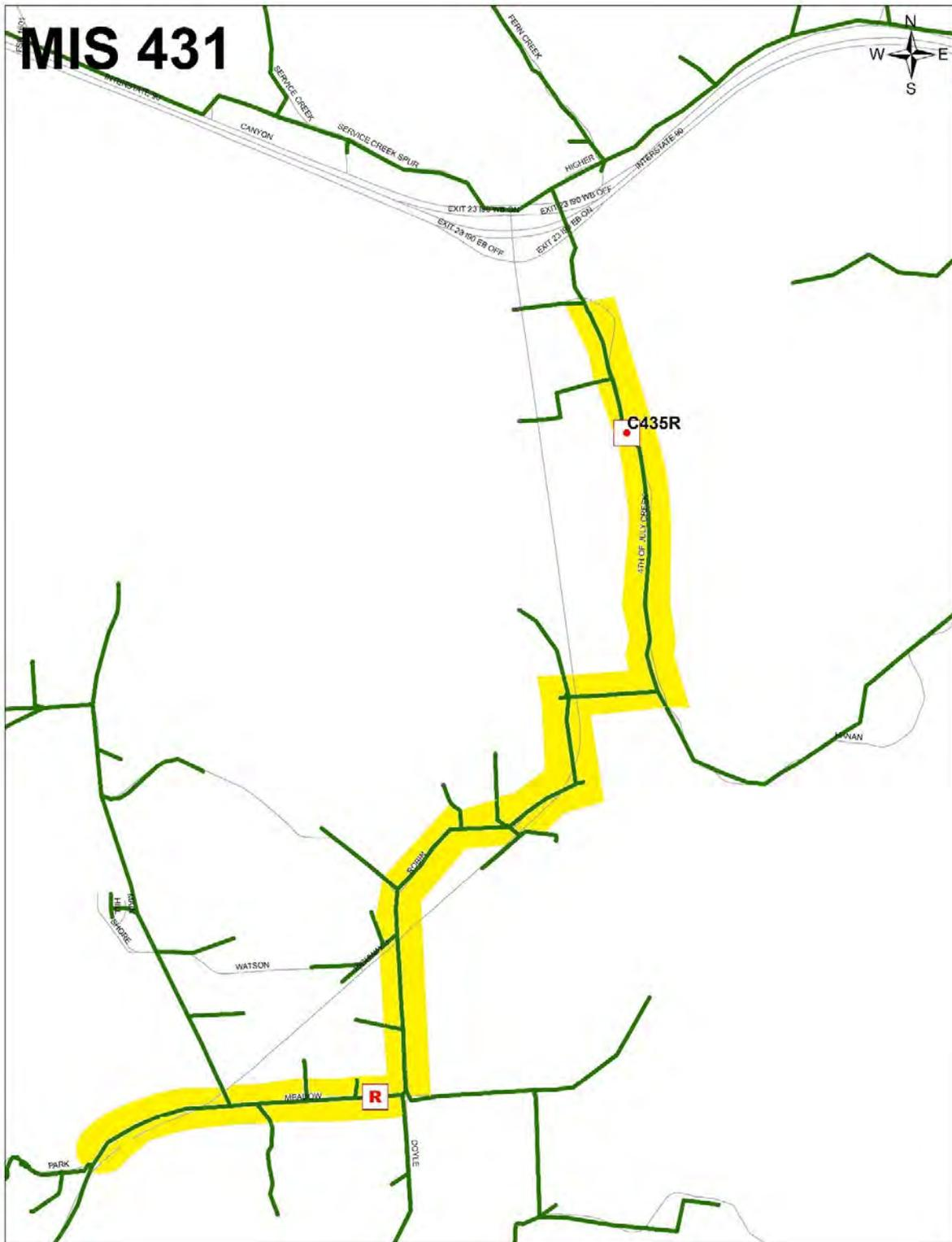
Figure 7. Polygon 16 Feeder Trunk Reconductor to 2/0 ACSR
