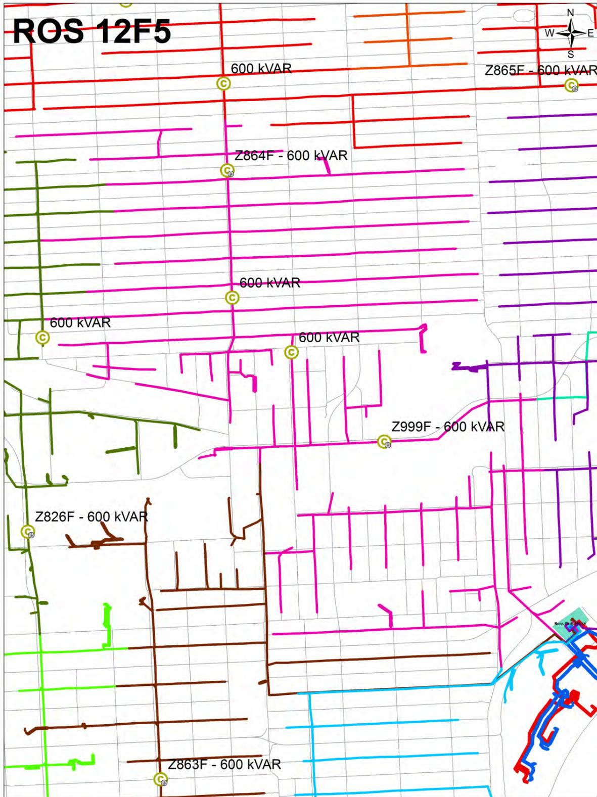
Figure 21. Existing Deployed Capacitor Banks on ROS 12F5
