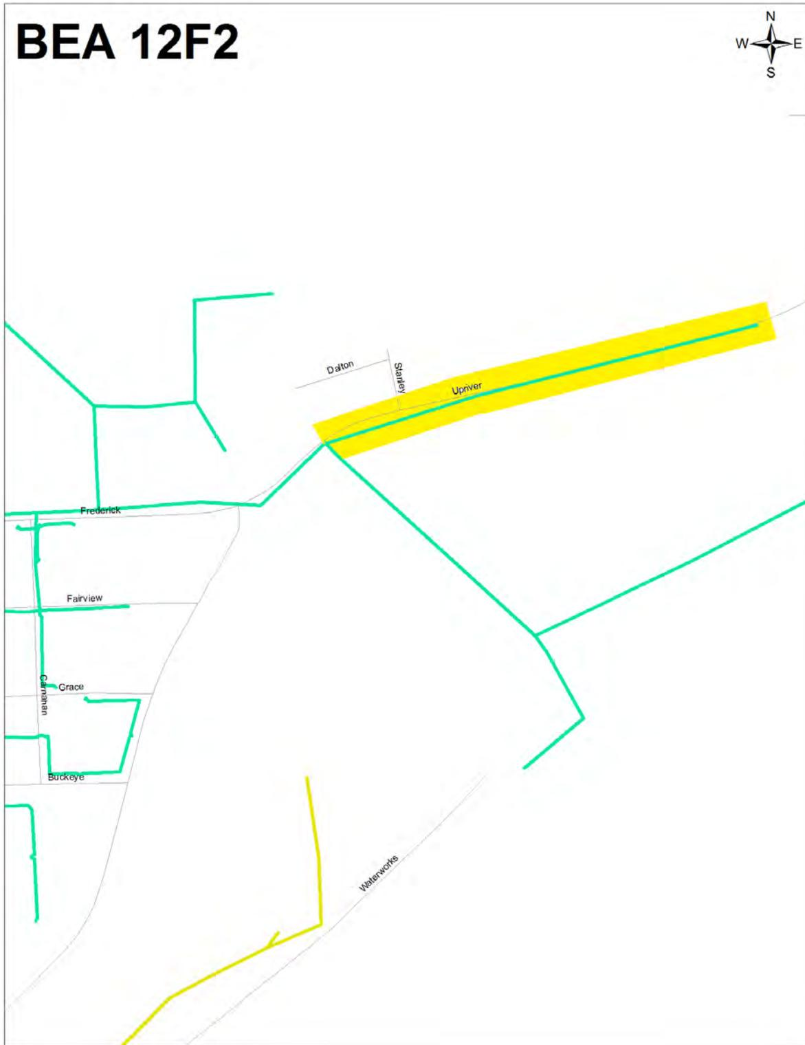
Figure 14. BEA 12F2 Primary Lateral Reconfiguration on Upriver
