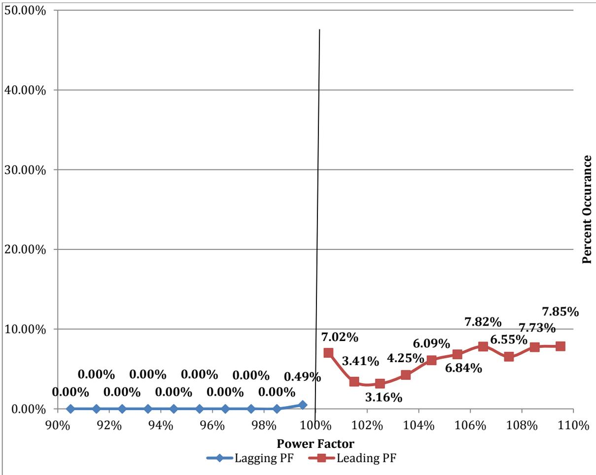
**Figure 12. Proposed Percent Occurance of Power Factor with 600 kVAR Removal**
