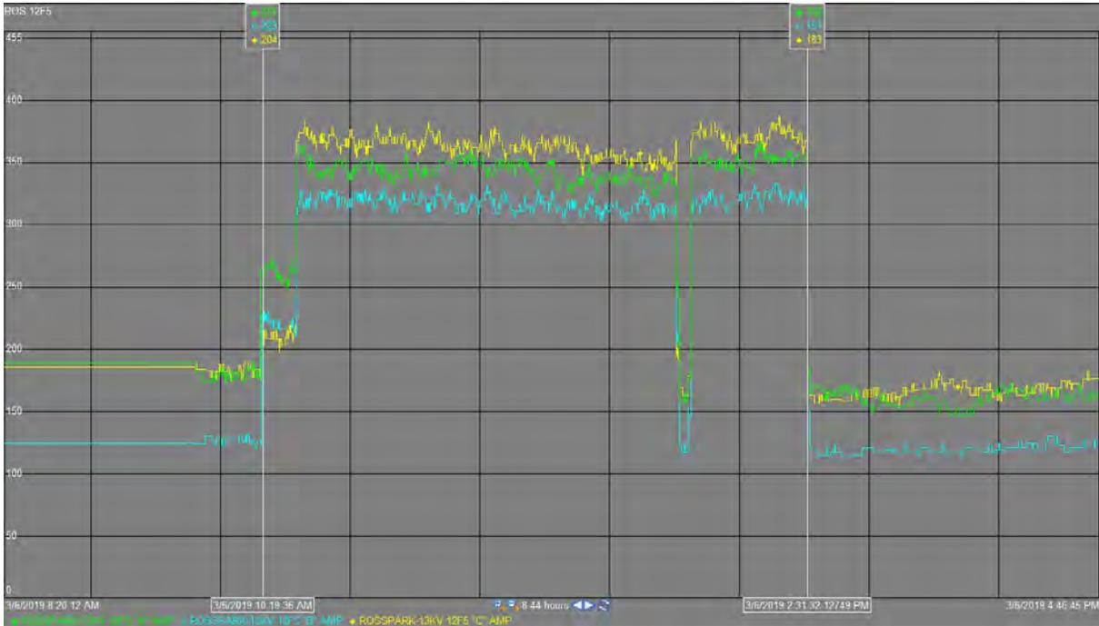
**Figure 9. ROS 12F5 Abnormal Feeder Configuration on 3/6/2019**
