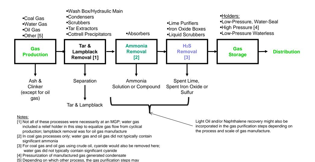
**Exhibit 2: Schematic Diagram of the Overall General Gas Manufacturing, Purification and Storage Processes**
