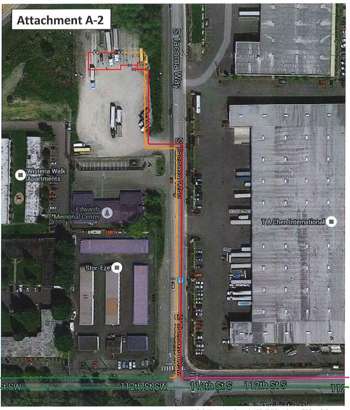
**I-5 Limit Station** Inlet/Outlet piping detail = 12" S Tacoma Supply #2 (250 psig -> 500 psig)
