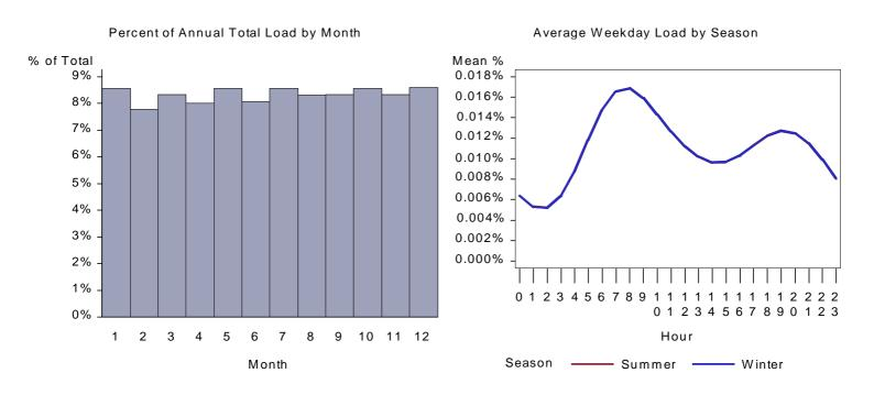
Figure 78. Utah Manufactured Water Heat Load by Month and Average Weekday
