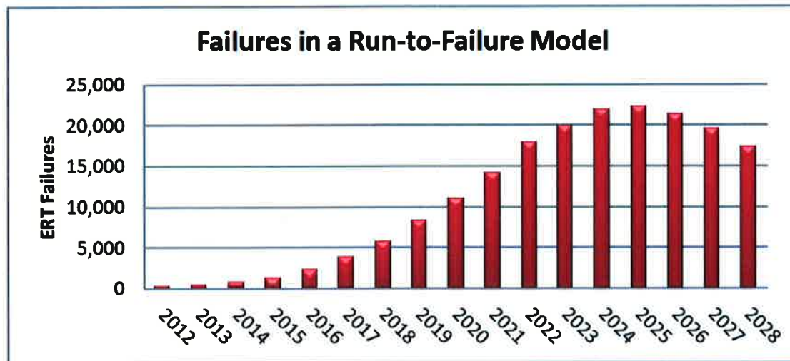
Figure 2 – Quantity of ERT Battery Failures per Year in Run-to Failure Model
