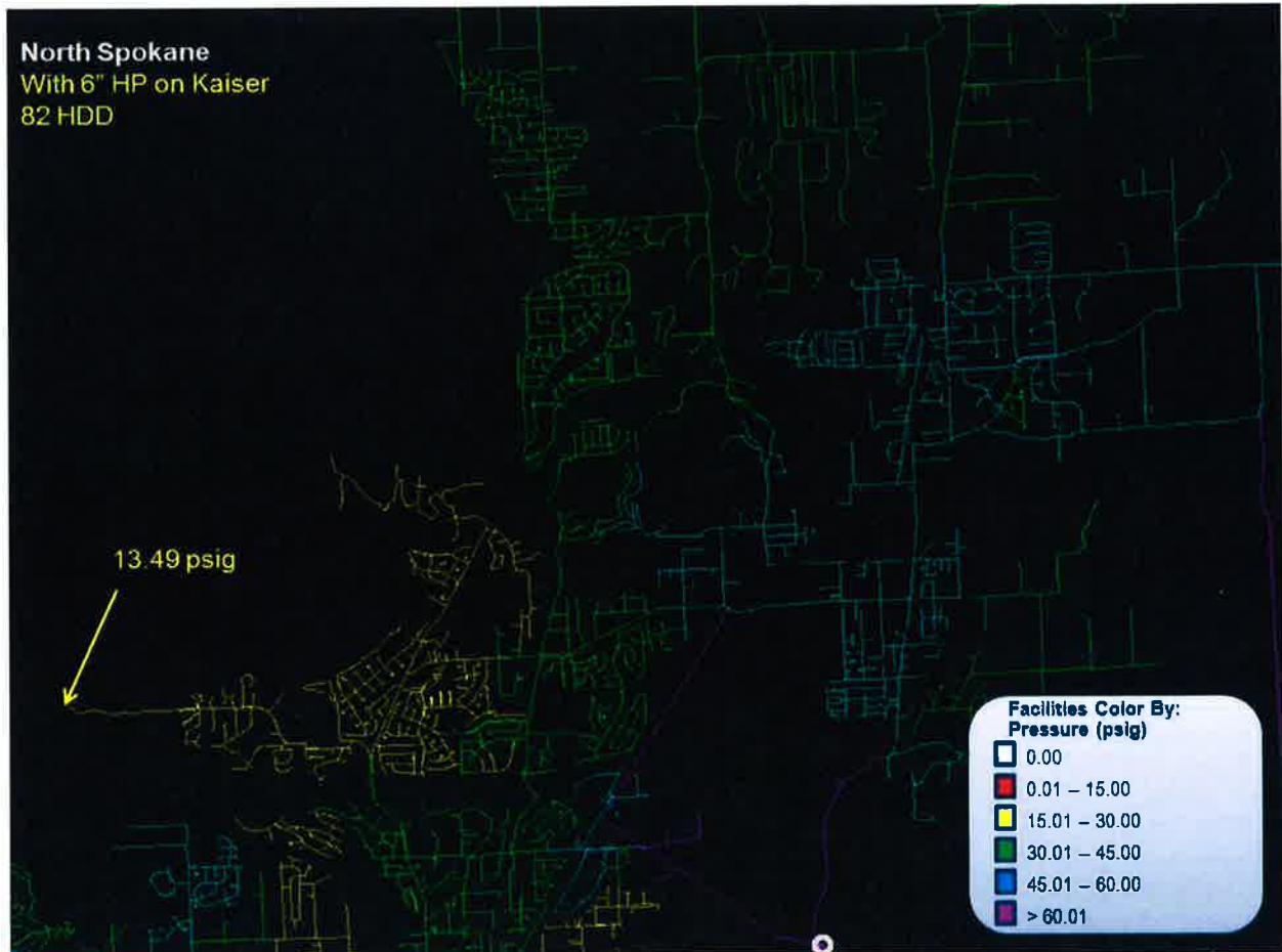
Image 2 – Distribution System Pressures after Proposed High Pressure Reinforcement (Option 2)
