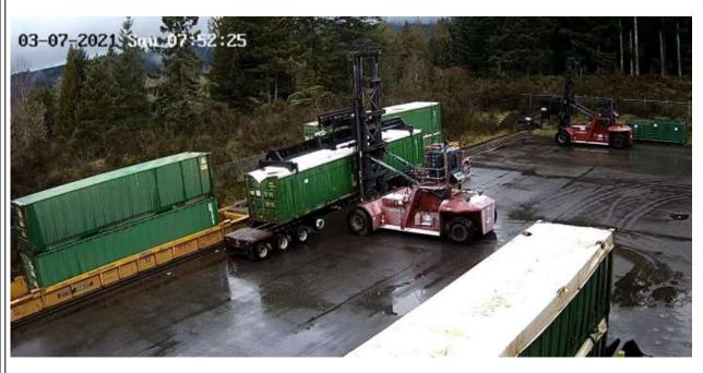
6.8 The photographs below show a closed intermodal container of OCC Rejects from PTP being offloaded from the truck to the UPRR train at NMF's rail spur, bound for WMDSO's Columbia Ridge Landfill in Oregon.
