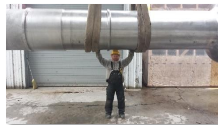
Cabinet Gorge turbine shaft
