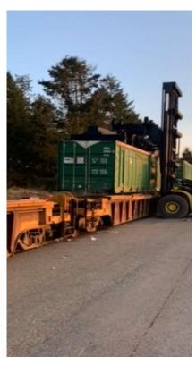
After loaded rail cars are switched to the PSAP rail line from either OVTS or NMF, the UPRR transports the intermodal containers to the Columbia Ridge Landfill in Oregon. WMDSO owns and operates the Columbia Ridge Landfill. Below is a photograph of a closed intermodal container of OCC Rejects being offloaded at the end of the COFC service from NMF's rail spur at the Columbia Ridge Landfill. Id. ¶ 8.
