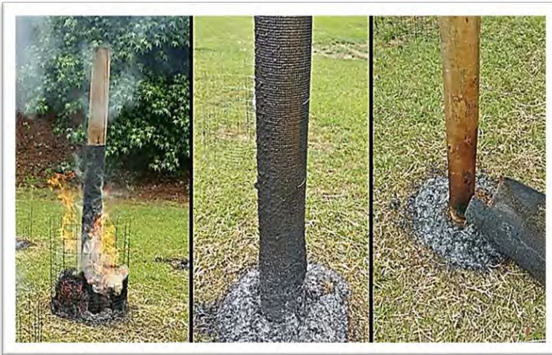
Figure 15. Fire resistant mesh wrap demonstration
