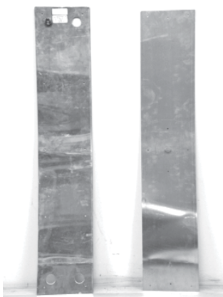
New Copper Ground Plate (MID 8969401) on Left and Current Model on Right
