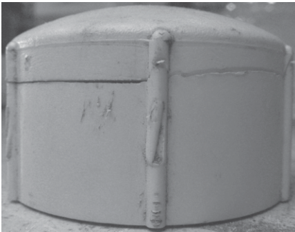
Cause Code D: Service Tee Cap with Damage from Overtorquing (wrench marks visible)
