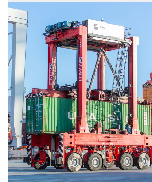
Automated straddle carriers at TraPac Terminal at the Port of Los Angeles.
