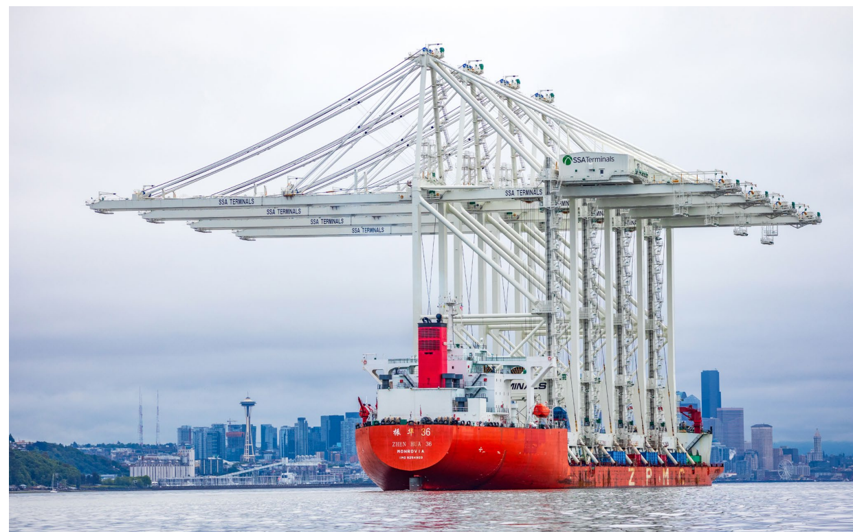
Four new Super Post Panamax Cranes arrive on the Zhen Hua 36 at SSA's Terminal 5 at the Port of Seattle.
