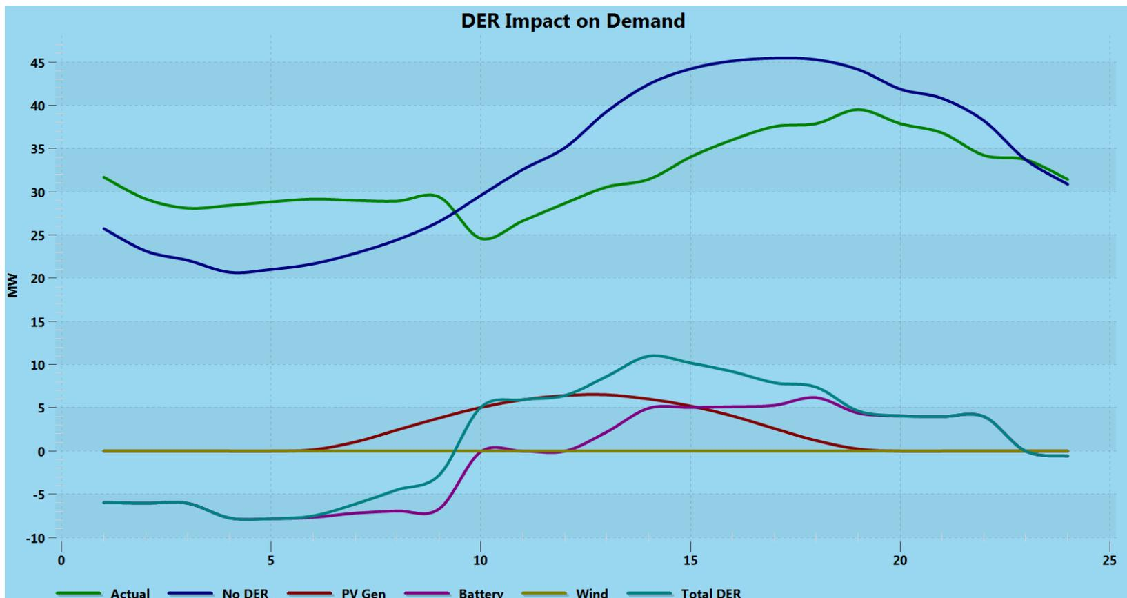
Assumes addition of 1.5 MW of solar per feeder or 9 MW total solar capacity.
