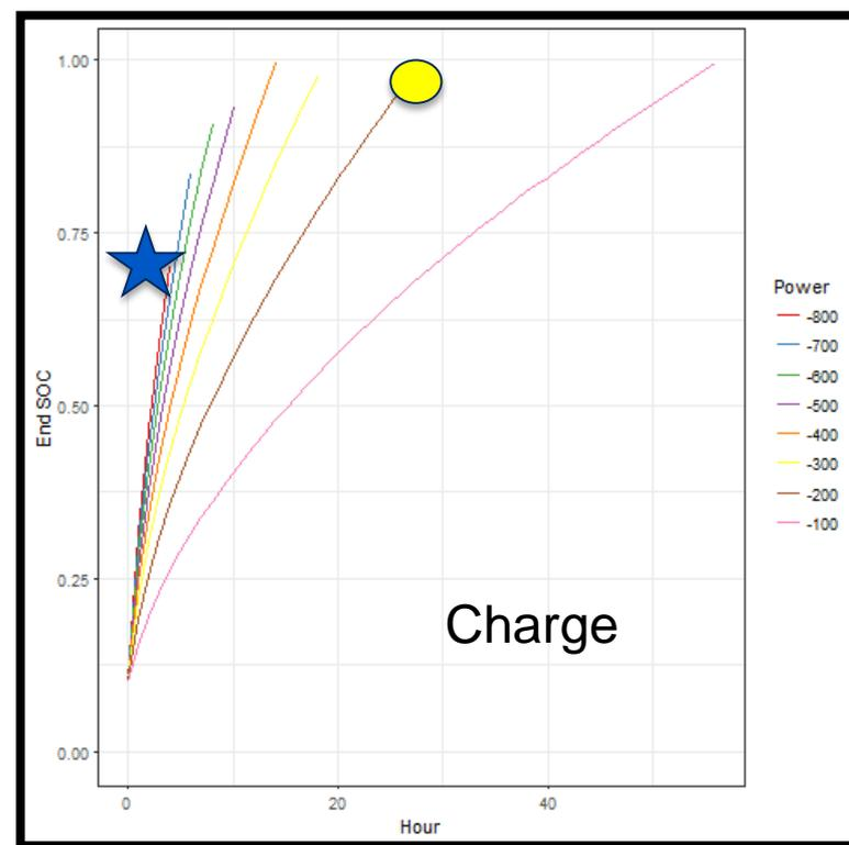
**State of Charge (SOC)** – An expression of the present battery capacity as a percentage of maximum capacity.
