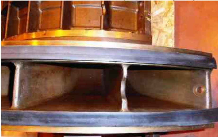
5 RS Generator Blower Stationary Blade Casting Gouges
