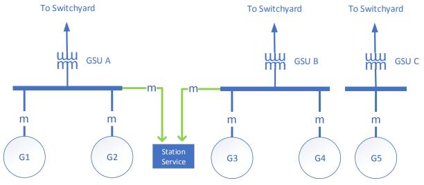
Figure 1 : Noxon Aggregate Registration with Unit Level Metering
