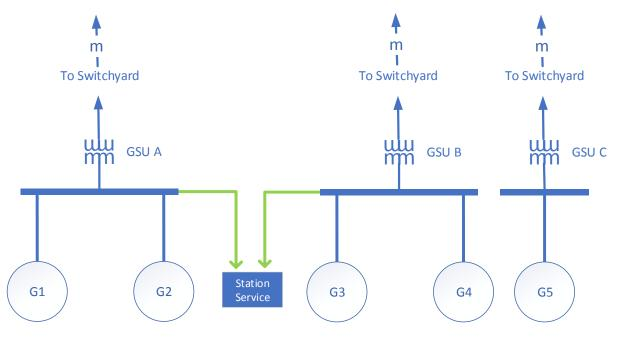
Figure 2: Noxon Aggregate Registration with High Side Metering
