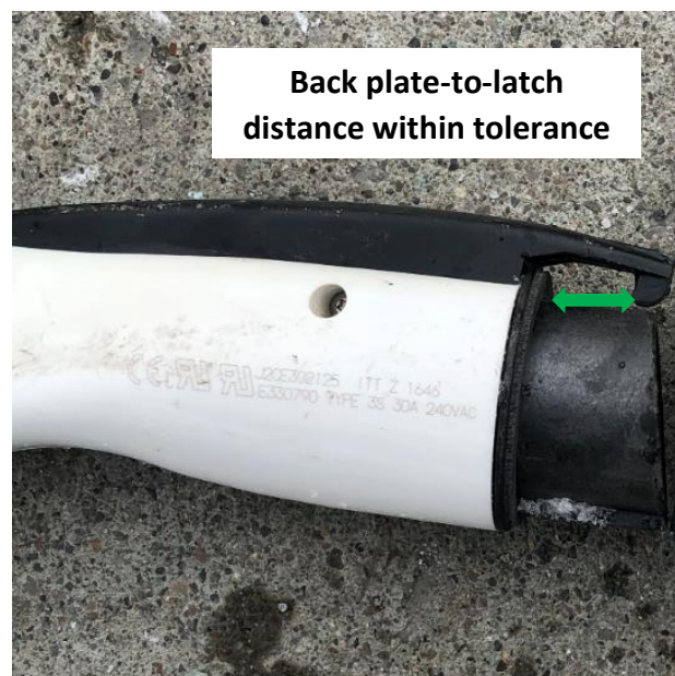
Figure 30. Example J1772 connector plate-to-latch tolerance
