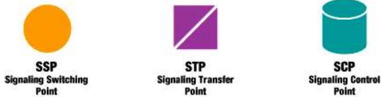
Figure 2. Signaling Network Elements
