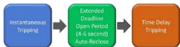
Base Level Fire Safety Mode
