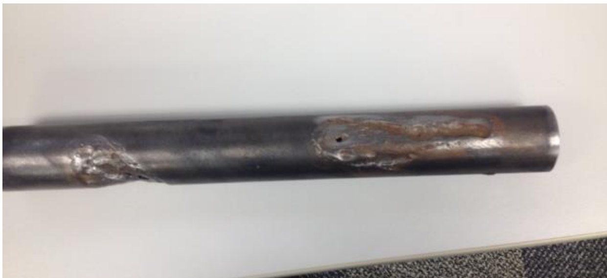
Image 1. Pipe Damage from Fault Incident
