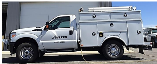
Avista electric service truck being charged
