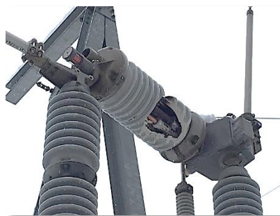
Above: Warden Switching Station failed PT Left: Circuit switch failure at Gifford Sub
