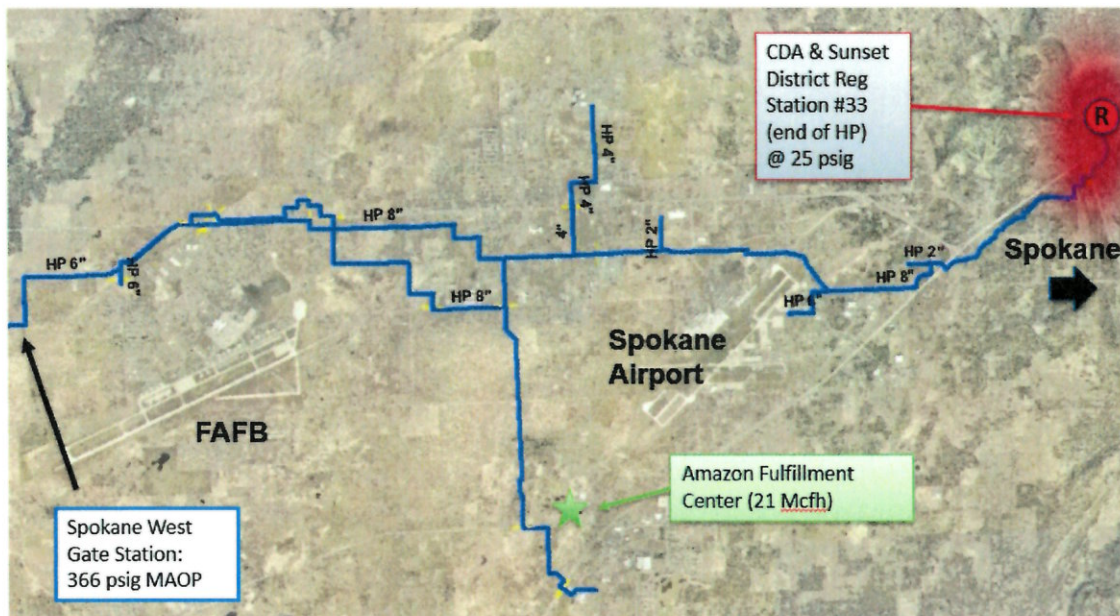
Image 1 – HP System as is, end of HP system at 25 psig
