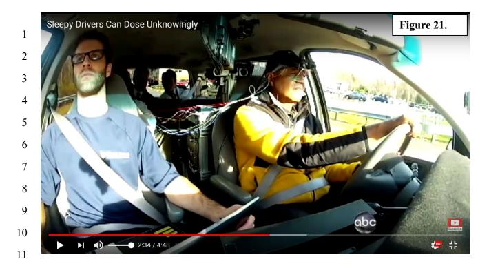
Figure 21. ABC News correspondent Mr. Ronald driving a specially instrumented van during a test driving session while outfitted for polysomnographic recording and eye tracking equipment. Investigator-observer in the front passenger seat can activate emergency braking maneuvers to prevent a crash. Seated in the second row, Dr. Charles Czeisler and Dr. Michael Lee are monitoring Mr. Claiborne's electroencephalogram and electrooculogram during the drive.
