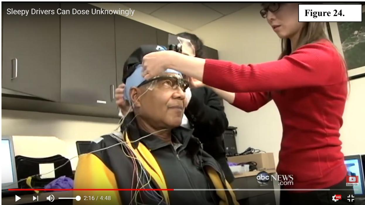
23 **Figure 24.** Polysomnographic (PSG) recording equipment used to monitor the electroencephalogram (EEG) and
