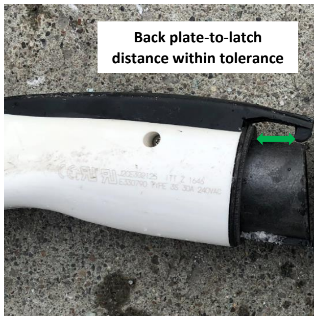
Figure 30. Example J1772 connector plate-to-latch tolerance
