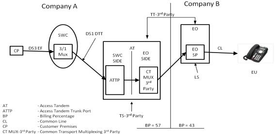
DTT - Direct Trunked Transport EF - Entrance Facility EO - End Office EO SP - End Office Shared Port EU - End User - Local Switching LS MUX - EF Multiplexer
