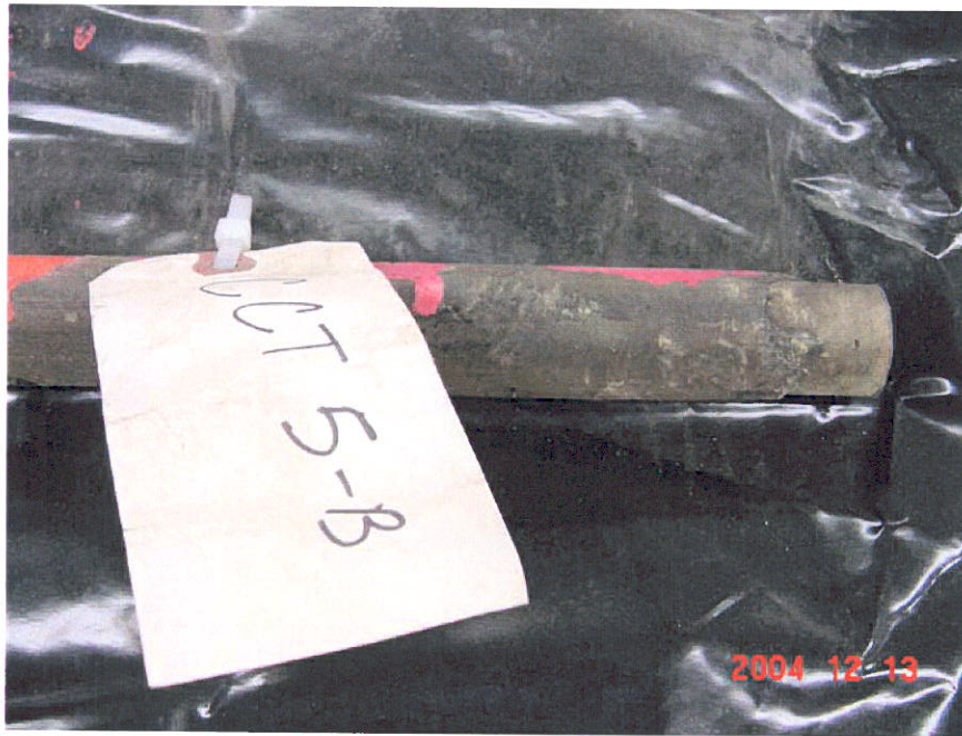
Figure 18. Photograph of unwrapped Segment 5 showing the downstream side of the pipe, CCT 5-B.
