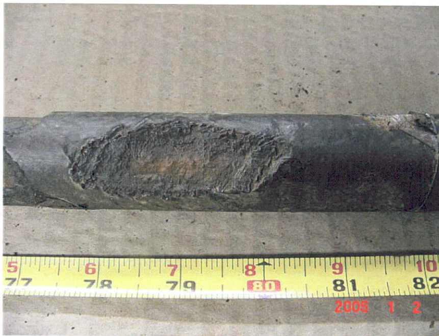
Figure 36. Photograph of Segment 10 showing a 2-inch long gouge to bare metal in the coating at the 78-inch location.
