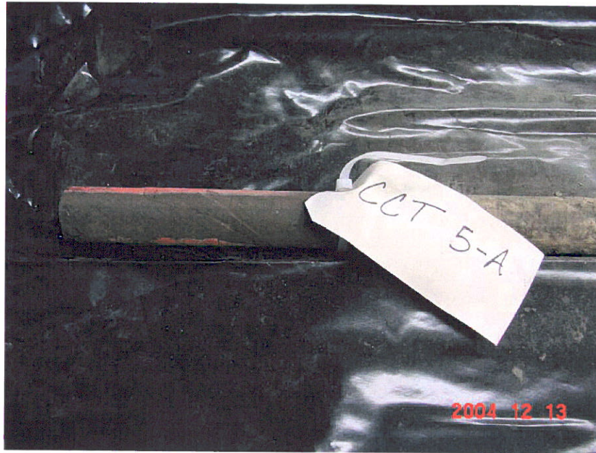
Figure 17. Photograph of unwrapped Segment 5 showing the upstream side of the pipe, CCT 5-A.
