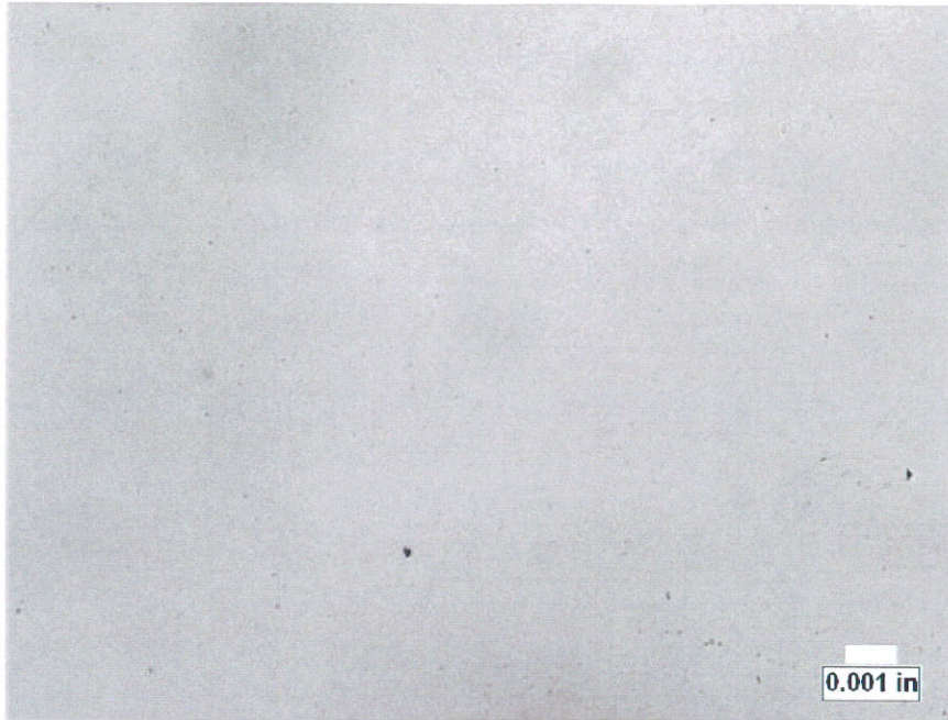
Figure 21. Light photomicrograph of as-polished Mount 9-B removed from maximum wall loss, taken at 200X.
