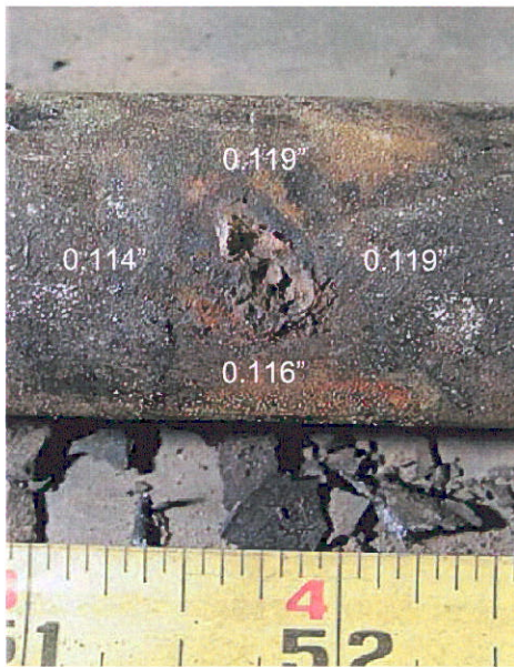
Figure 4. Circumferential profile of the anomaly at the 49.75-inch location of Segment 4.
