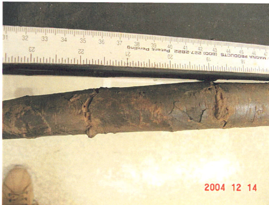
Figure 34. Photograph of Segment 10 showing an example of the coating deformations that occurred on the extrados of the bend.
