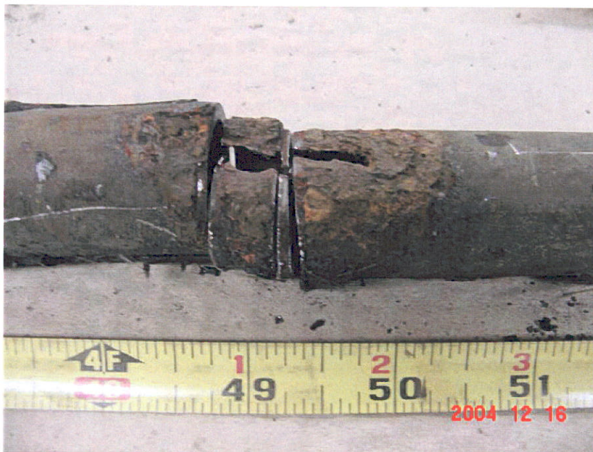
Figure 8. Photograph of Segment 10 showing where Mount 10-4B (2 nd piece from left) and Surface 10-4C (3 rd piece from left) were cut out of the pipe.
