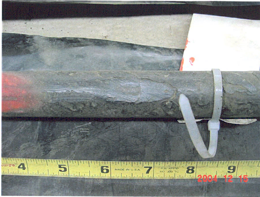
Figure 15. Photograph of Segment 7 showing a gouge in coating from the 6-inch location to the 7.5-inch location.
