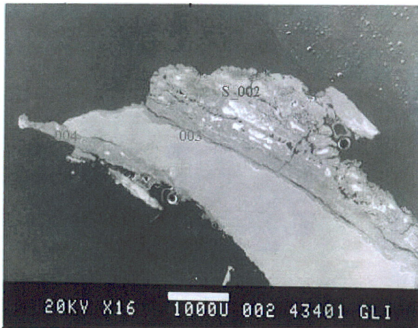
Figure 10. SEM photomicrograph 002 of Mount 10-4B showing the debris on the OD of the penetration plus the locations of photomicrographs 003 and 004 and EDS scan S-002.
