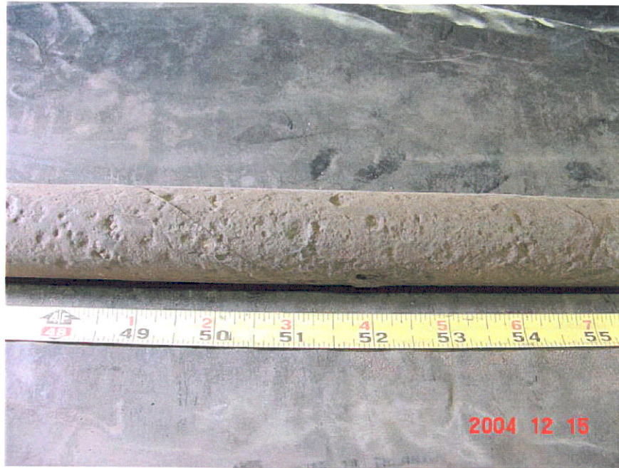
Figure 11. Photograph of Segment 5 showing an area of coating deformations that extended from the 45-inch location to the 62-inch location.
