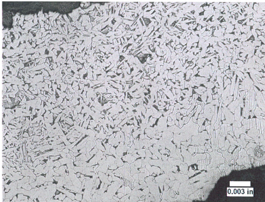
Figure 22. Light photomicrograph of etched Mount 10-4B microstructure near wall loss, taken at 100X.
