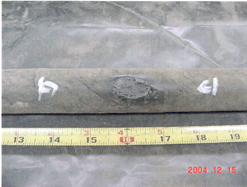
Figure 25. Photograph of Segment 9 showing a 1-inch deformation in the coating at the 16-inch location.
