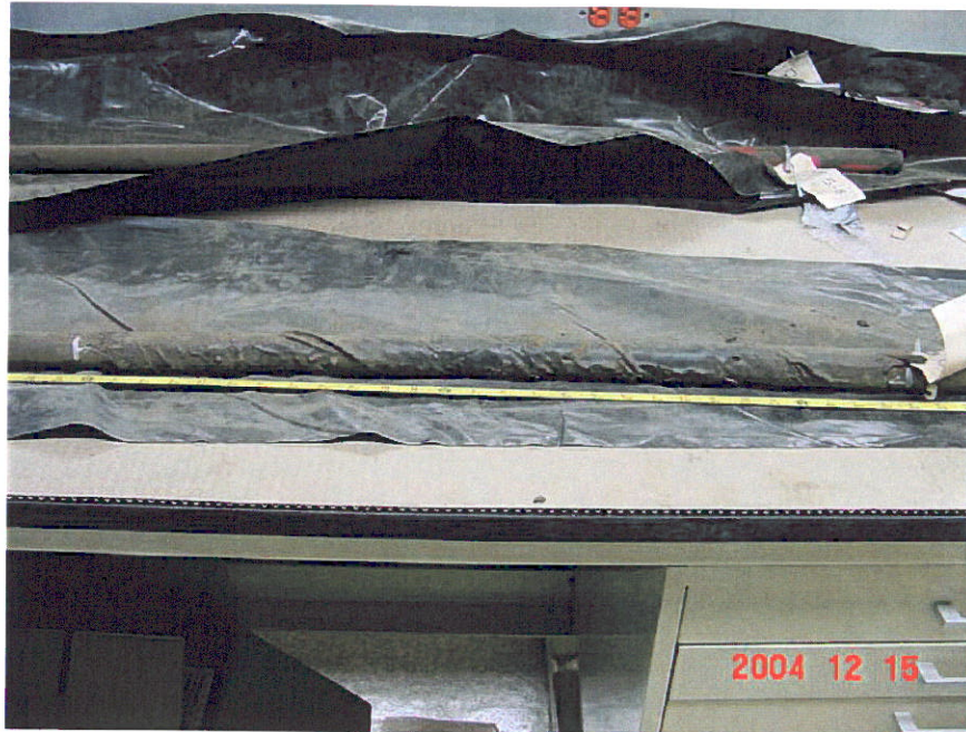
Figure 9. Photograph of Segment 4 showing a field applied outer wrap that covered the pipe between the 60.5-inch to 88-inch locations.
