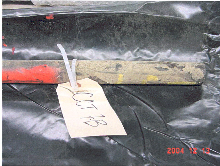
Figure 25. Photograph of unwrapped Segment 7 showing the downstream side of the pipe, CCT 7-B.
