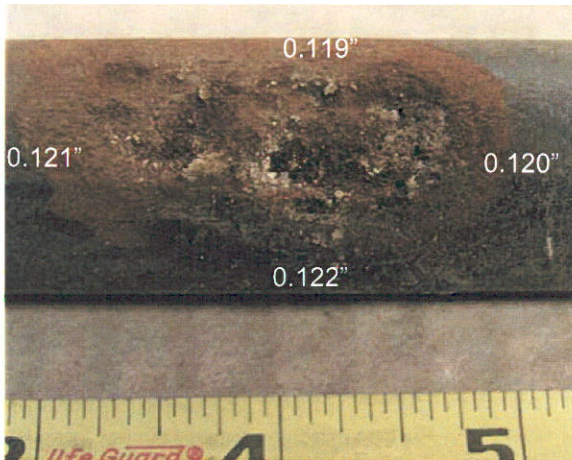
Figure 1. Circumferential profile of the anomaly at the 4-inch location of Segment 1.
