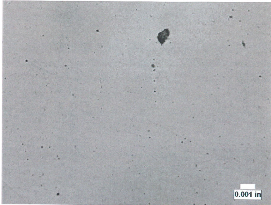
Figure 3. Light photomicrograph of the as-polished Mount 1-B away from the area of wall loss of taken at 200X.
