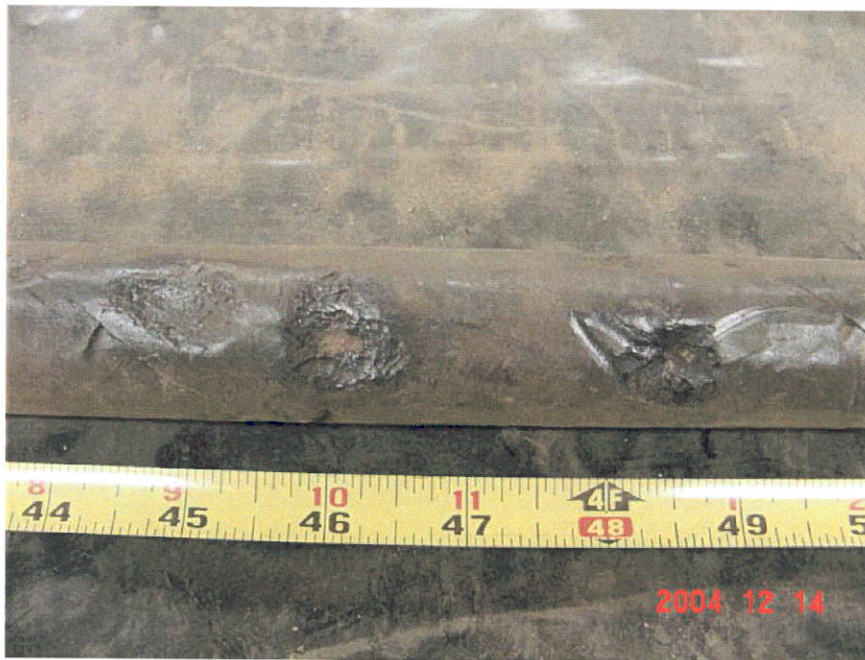
Figure 24. Photograph of Segment 8 showing two of the coating deformations to bare metal.
