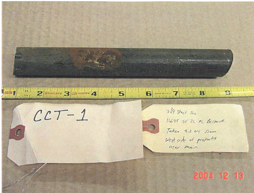
Figure 1. Photograph of Segment 01 showing the pipe as-received had little remaining coating.
