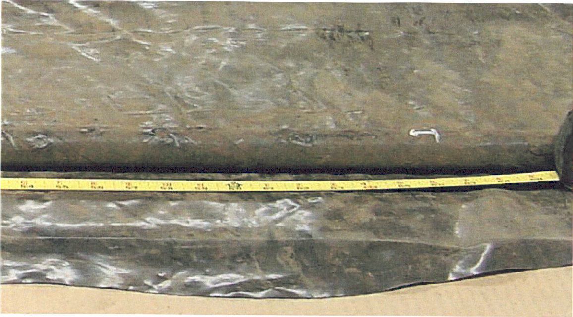
Figure 23. Right side of the photograph in Figure 21 showing a coating deformation at the 57.75-inch location
