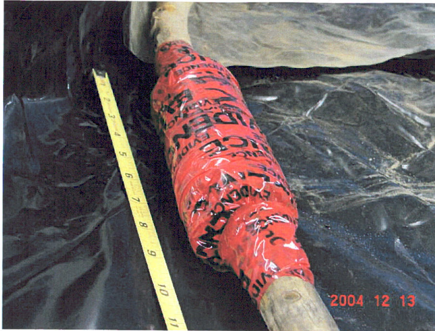
Figure 37. Photograph of unwrapped Segment 10 showing red evidence tape on a protective covering on the pipe.
