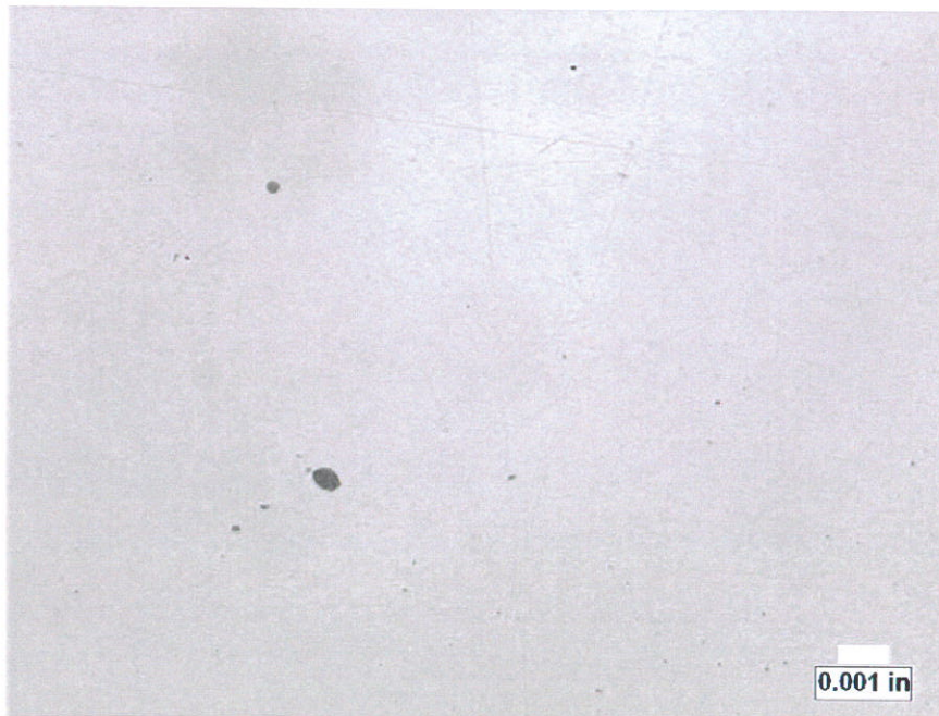
Figure 8. Light photomicrograph of as-polished Mount 4-B removed from maximum wall loss, taken at 200X.
