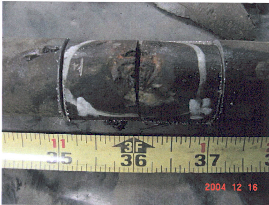
Figure 6. Photograph of Segment 9 showing where Mount 9-B (2 nd piece from left) was cut out of the pipe.
