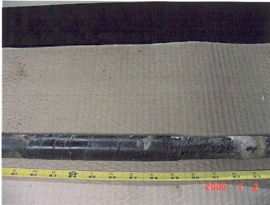
Figure 37. Photograph of Segment 10 showing a "transition" coating between the 82 to 93-inch locations.
