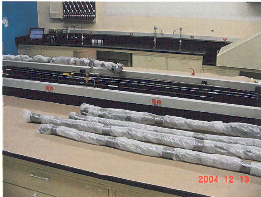
Figure 4. Photograph of pipe Segments 6 through 9 with Segment 10 in the background showing how the individual pipes were wrapped individually in the shipping crate.
