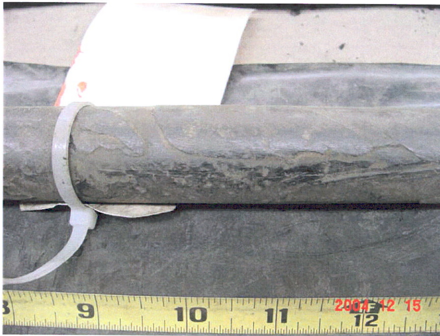
Figure 16. Photograph of Segment 7 showing scratched coating from the 7-inch location to the 19-inch location.
