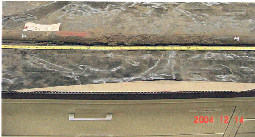
Figure 20. Photograph of Segment 8 showing a coating wrap located between the 6-inch to 29-inch location.
