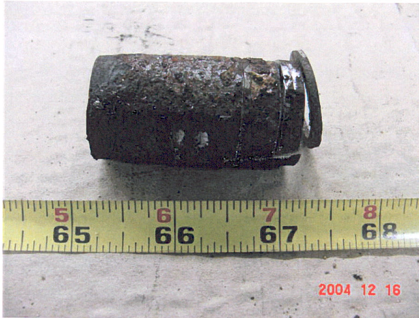
Figure 9. Photograph of Segment 10 showing where Surface 10-5B-2 (last piece on right) was removed from the pipe.
