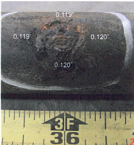
Figure 6. Circumferential profile of the anomaly at the 36-inch location of Segment 9.
