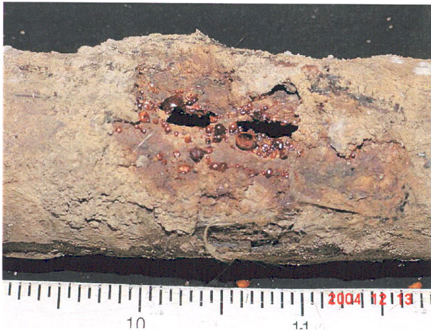
Figure 32. Photograph of Segment 10 showing a 1-inch through wall indication at the 48-inch location with granules around the indication.
