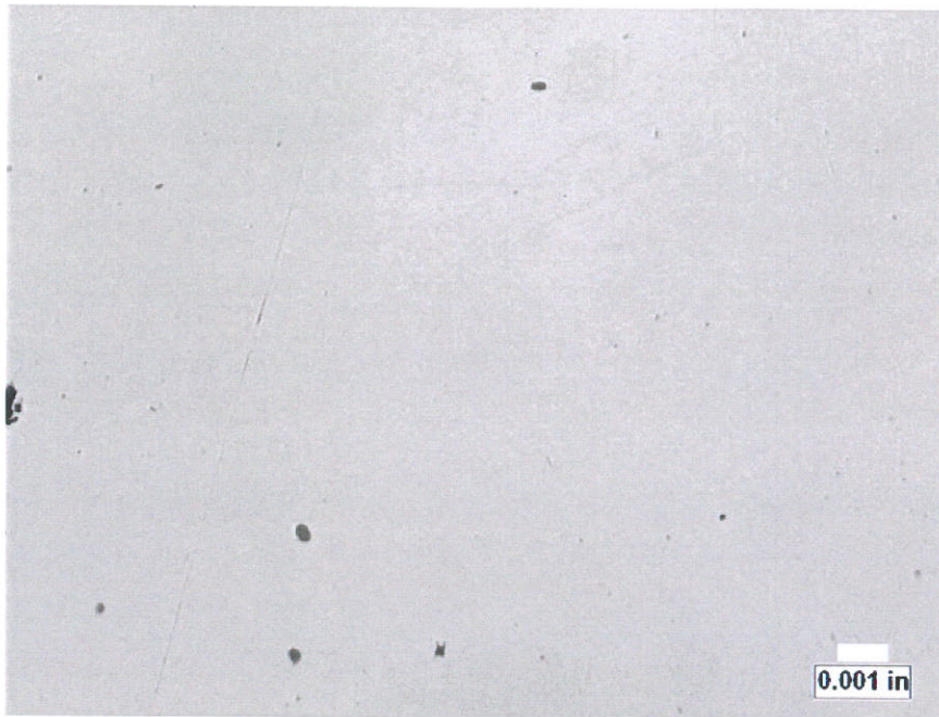
Figure 7. Light photomicrograph of as-polished Mount 4-B near maximum wall loss taken at 200X.
