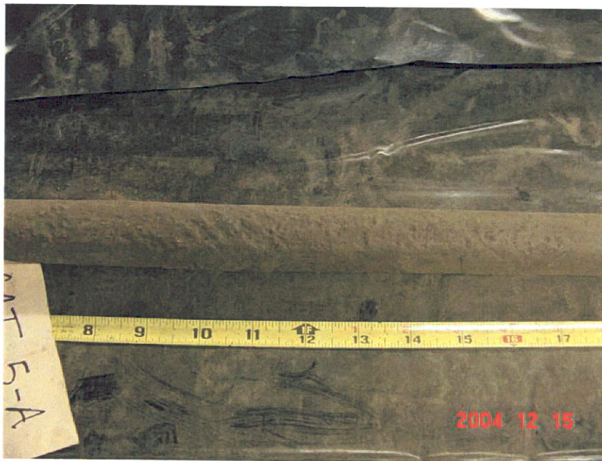
Figure 10. Photograph of Segment 5 showing an area with coating deformations that extended from the 5-inch location to the 19-inch location.
