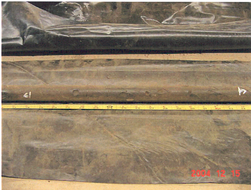
Figure 26. Photograph of Segment 9 showing an area of scratches and dents in the coating between the 21-Inch location and the 34-inch location.
