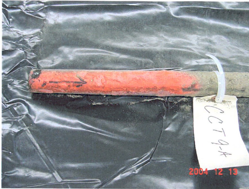
Figure 31. Photograph of unwrapped Segment 9 showing the upstream side of the pipe, CCT 9-A.
