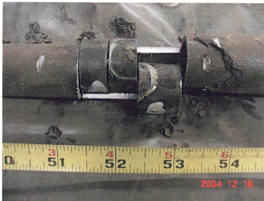
Figure 4. Photograph of Segment 4 showing where Mount 4-B (3rd piece from left) was cut out of the pipe.
