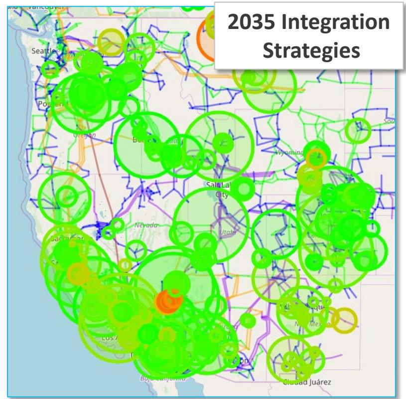
Integration Strategies scenario included substantive transmission builds in California, Colorado, New Mexico, Wyoming/Utah, and Montana, with minor upgrades in the rest of the NW region
