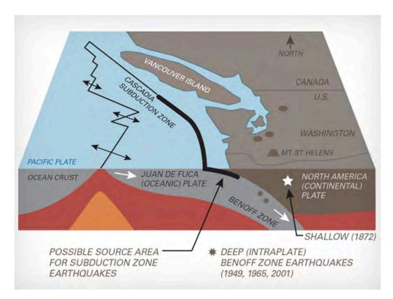
Figure A: Cross Section of the Cascadia Subduction Zone (Source: Washington State Department of Natural Resources)
