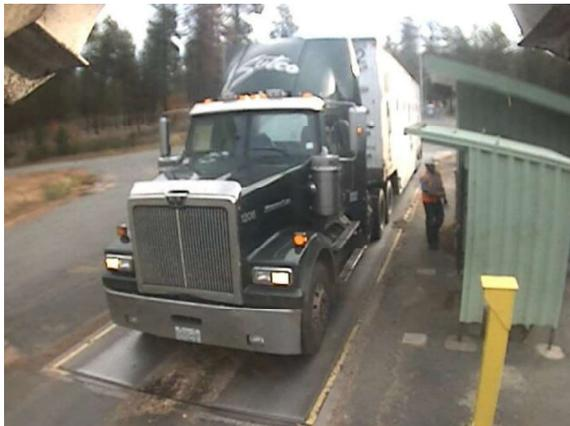
*Truck was intentionally positioned short on the scale.*
