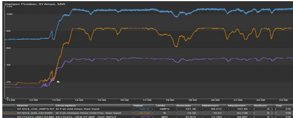
The graph above shows a typical instance of the plant ramping up to nearly full load (MWs shown in purple) with the damper position maxing out (orange trend) as the motor tops out in amperage (shown in blue). Once the amps on the motor plateau around 105 amps, the other parameters are forced to plateau as well. This shows how the motor can be a limiting factor in the plant's MW output.
