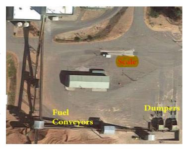
**Fuel Conveyors** - Fuel conveyers move the fuel from the truck dumpers to a metal detection system, then to the fuel hog system and finally out to the fuel yard.
