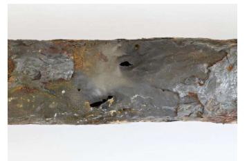
need to be taken offline immediately but can sometimes run for a few weeks until the best economic opportunity allows for the shutdown to be scheduled. If the unit is left running with a superheater tube leak the steam blowing from the tube may hit an adjacent tube steam cut through the metal and create another tube leak. The random thinning and scale make it impossible to predict when and where the next tube leak will occur.
