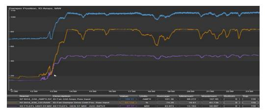
The graph above shows a typical instance of the plant ramping up to nearly full load (MWs shown in purple) with the damper position maxing out (orange trend) as the motor tops out in amperage (shown in blue). Once the amps on the motor plateau around 105 amps, the other parameters are forced to plateau as well. This shows how the motor can be a limiting factor in the plant's MW output.
