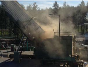
After the load is raised into the air and the fuel is discharged out of the back of the haul trailer into the truck receiving hopper a large plume of dust often launched into the air and
