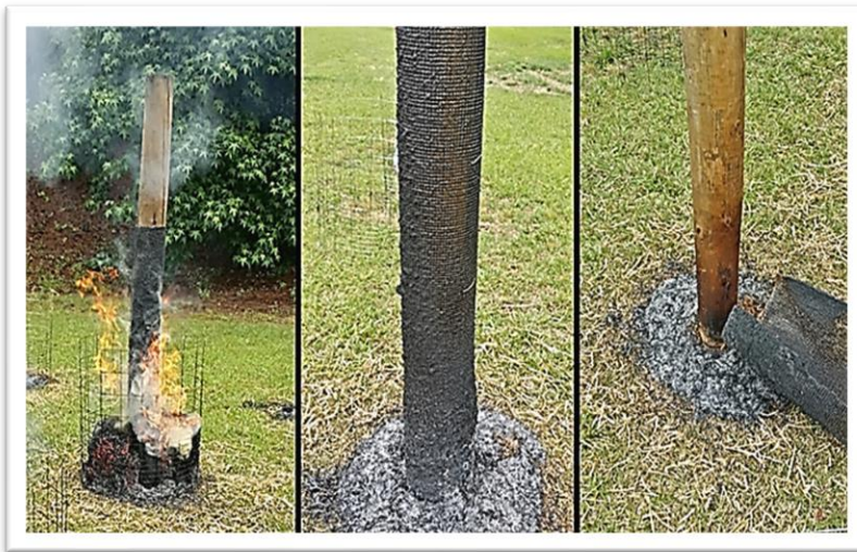
Figure 15. Fire resistant mesh wrap demonstration
