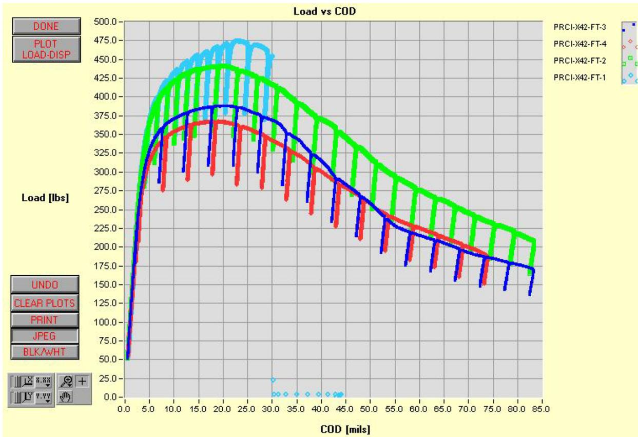
Fig. E3 Example of load versus crack opening displacement (COD) data from the disk compact specimens of the X42 pipeline steel material. Specimen Number “PRCI-X42-FT-1” cleaved since it was tested at -118°F. The other three specimens were tested at room temperature.
