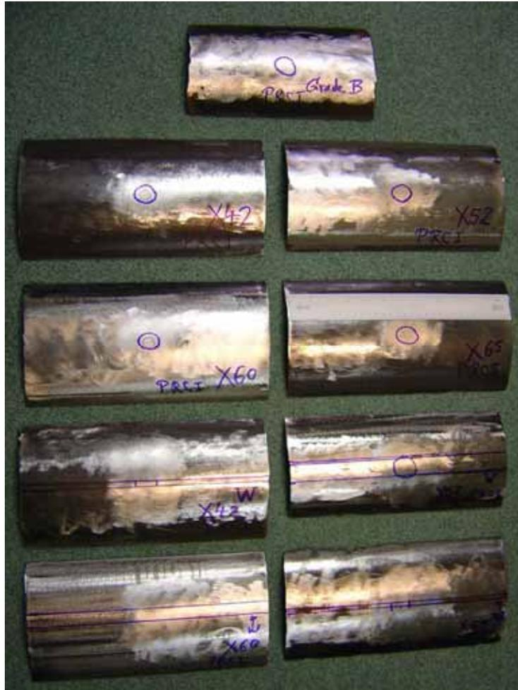
Fig. 8 Photo of all 9 pipeline sections (Grade B base metal, X42 BM, X52 BM, X60 BM, X65 BM, X42 W, X52 W, X60 W, and X65 W).
