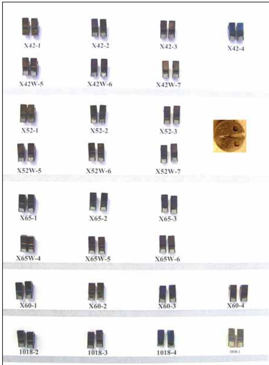
Fig. 16 Fracture surfaces of all disk compact fracture toughness specimens from the base metal and seam welds of several pipeline steels and from 1018 steel plate. The 1018 steel material was used before obtaining Grade B pipeline material.
