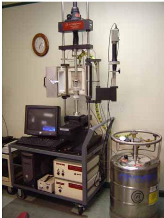
Fig. 2 The bench-top SSM system (Model SSM-B4000) is shown above with all optional accessories including an environmental chamber for low and high temperature testing. ATC's patented SSM systems have been in use worldwide since 1991. In addition to performing the innovative ABI tests, the bench-top systems are also state-of-the-art universal testing machines that perform destructive tensile and fracture toughness tests.
