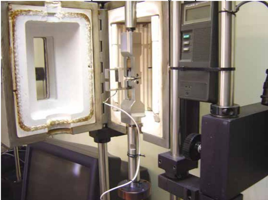
Fig. 6 Destructive fracture toughness testing setup using the environmental chamber of the bench-top SSM system (Model SSM-M4000).
