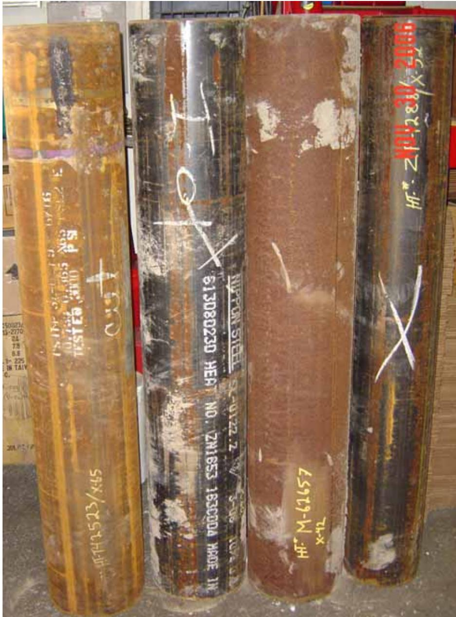
Fig. 7 Photo of the four pipelines received from Shell (grades X42, X52, X60, and X65).
