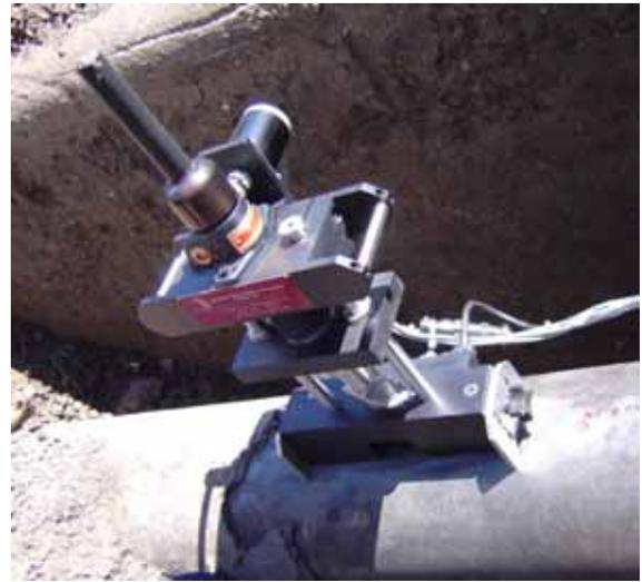
Fig. 1 The testing head of the miniature SSM system (Model SSM-M1000) is mounted using electric magnets on steel pipelines.
