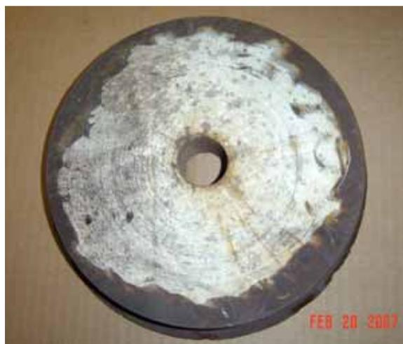
Fig. 9 Photographs of both surfaces of the 9-inch diameter steel trepan from a BP storage tank.
