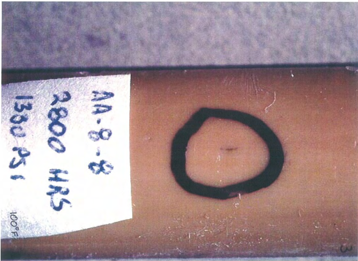
Figure 5 -- Slit fracture resulting from a stress rupture test conducted at 100 °F. Note lack of deformation visible in the fracture. This pipe was manufactured by DuPont in 1977. After failing Minnegasco's incoming inspection tests, the pipe was subjected to stress rupture testing. (Source: Henrich, R.C., and Funck, D.L., "Effects of ESCR Variation on Some Other Properties of Plastic Pipe." Proceedings, Eighth Annual Plastic Fuel Gas Pipe Symposium, 1983. )
