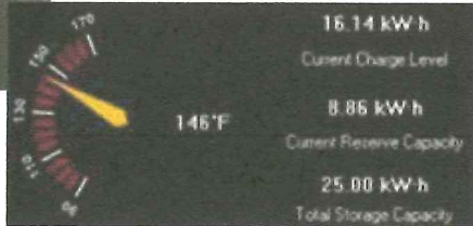
Below: Control panel available to grid operator showing available storage and total storage capacity in a water heater.
