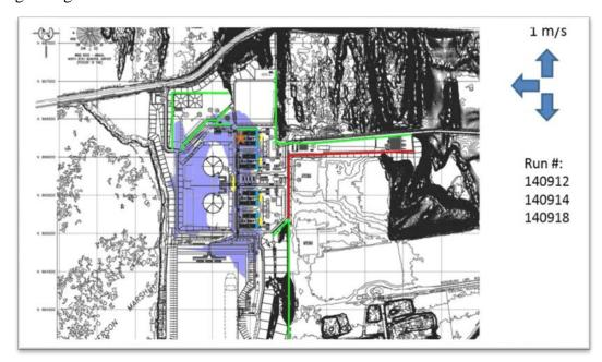
Figure 4.13.5 from DEIS LNG Spill from a Guillotine Rupture of the Ship Loading Header
