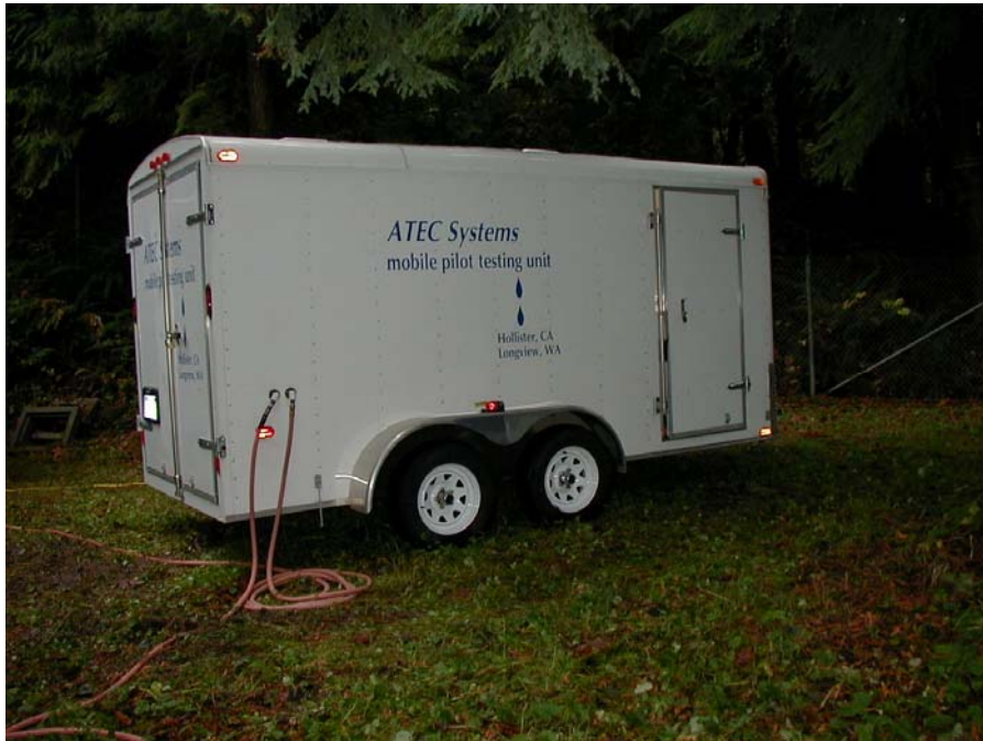
The exterior of ATEC Systems' pilot trailer is shown above. The source and product water connections are shown entering and exiting the trailer. Inside dimensions are 14' x 6' x 6½'.
