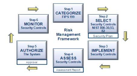
Step 1 of the life cycle involves categorization of the various systems involved in the Smart Grid projects, and is presently being performed by Avista. This categorization step performs an inventory of all the various systems, existing and future, which are involved in the Smart Grid implementation. An assessment is made of each system's impact regarding confidentiality, integrity, and availability and what the loss of any of the attributes would have on operations, assets, and individuals.
