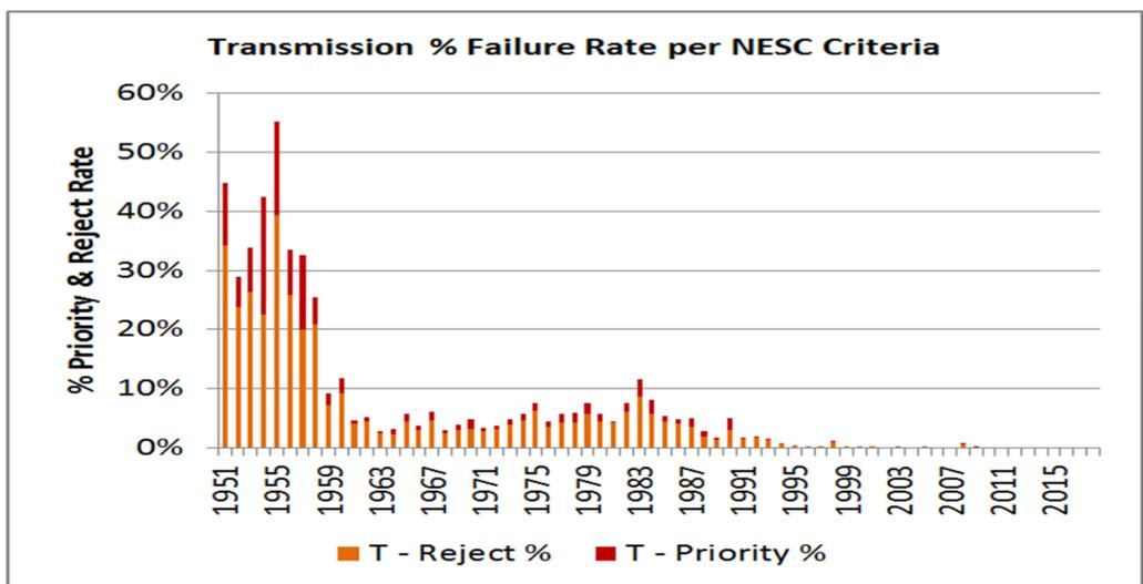
**Figure 6-1: Transmission Pole Failure Rate vs Install Date**
