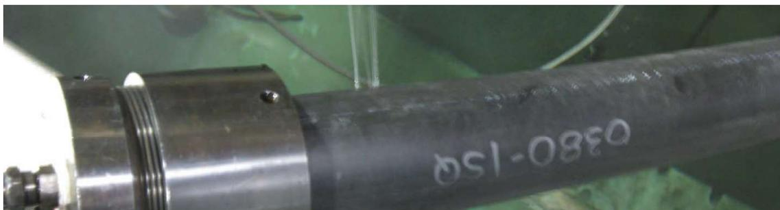
**Slit Failure in Specimen 131837-061 (0380-1SQ) Tested at 176°F/98 psig**
