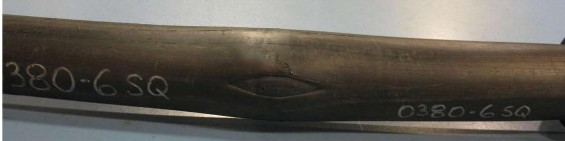
**Ductile Failure in Specimen 131837-066 (0380-6SQ) Tested at 73°F/355 psig**
