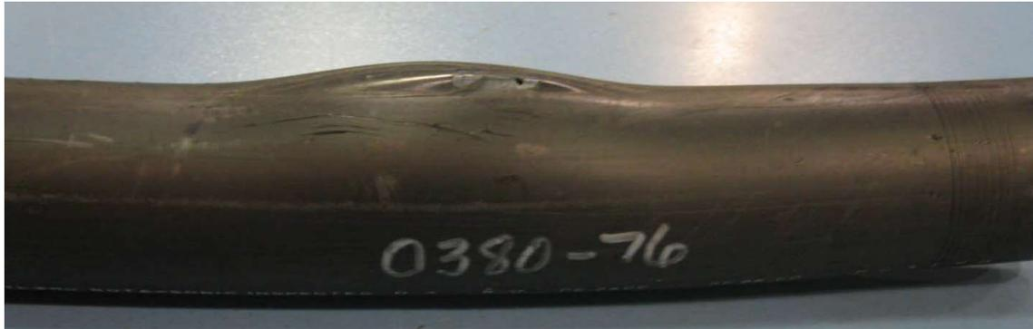
**Ductile Failure in Specimen 131837-025 (0380-76) Tested at 73°F/355 psig**
