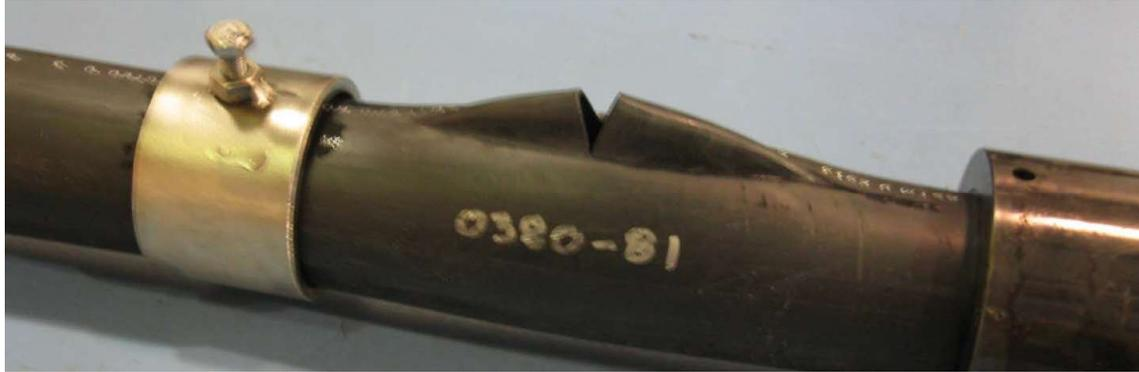
**Ductile Failure in Specimen 131837-054 (0380-81) Tested at 73°F/337 psig**
