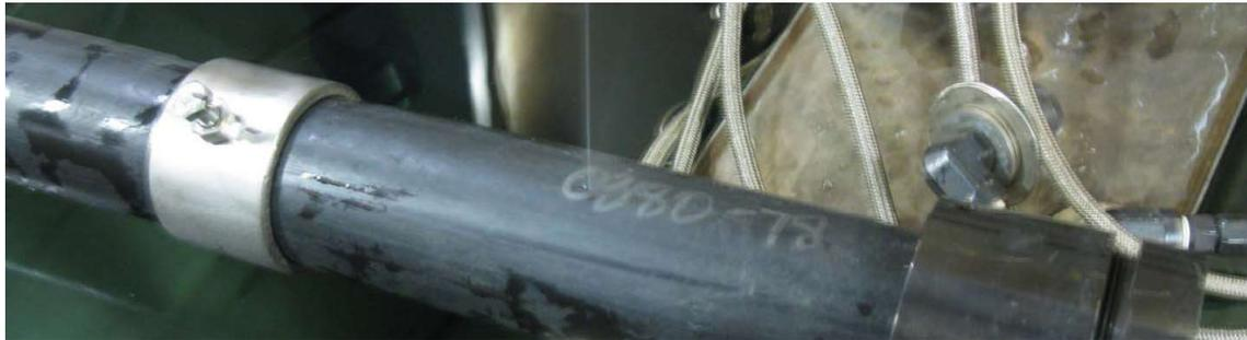
**Slit Failure in Specimen 131837-027 (0380-78) Tested at 140°F/220 psig**
