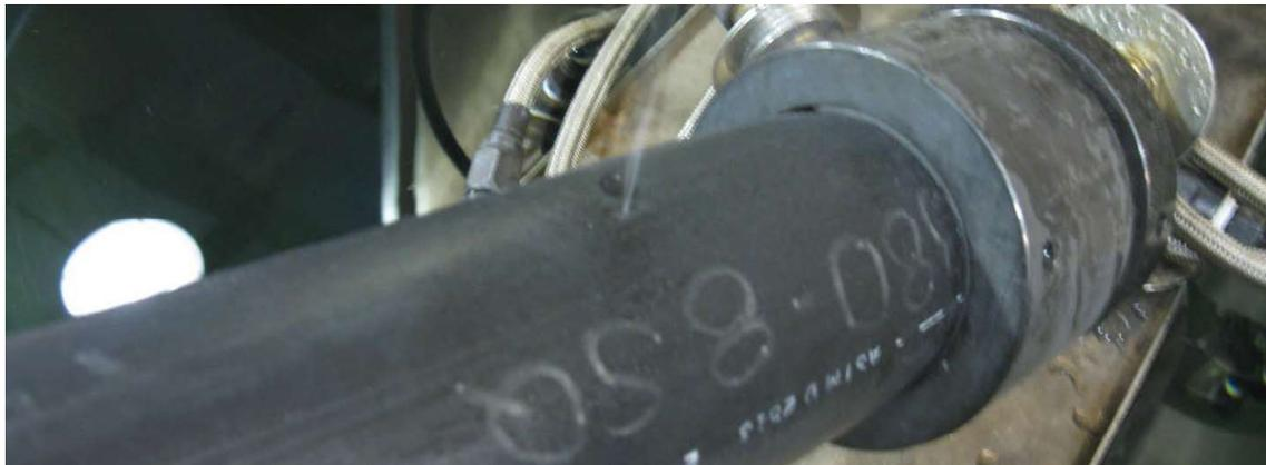
**Slit Failure in Specimen 131837-080 (0380-8SQ) Tested at 140°F/200 psig**
