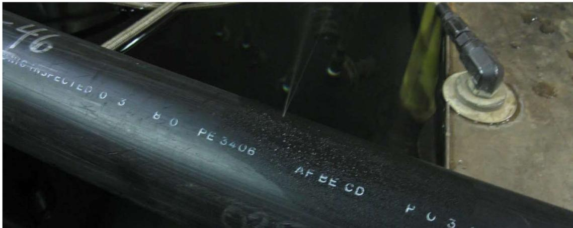
**Slit Failure in Specimen 131837-036 (0380-46) Tested at 140°F/220 psig**
