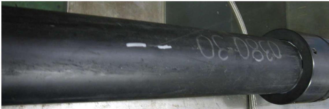
**Slit Failure in Specimen 131837-005 (0380-30) Tested at 176°F/120 psig**
