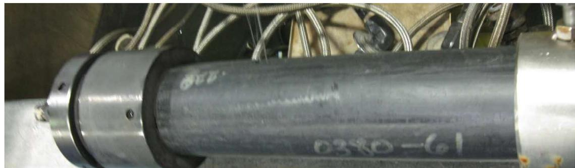
**Slit Failure in Specimen 131837-051 (0380-61) Tested at 176°F/100 psig**
