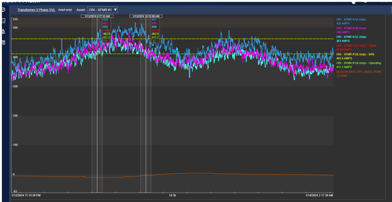
Figure 17: Orin 115/13kV Transformer 1 loading January 13, 2024
