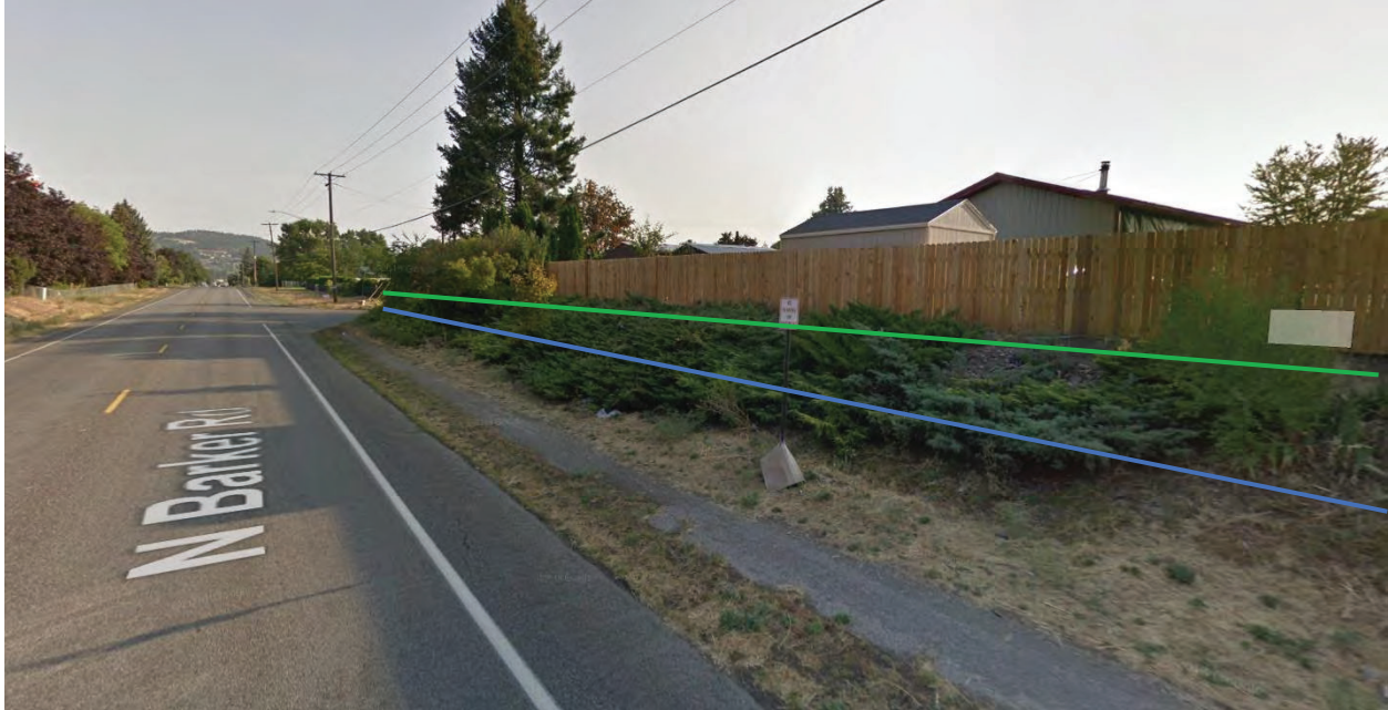
18710 East Marlin Drive as seen from Barker Road heading north. The blue line represents the approximate sidewalk edge and the green line represents the approximate existing ROW line.
