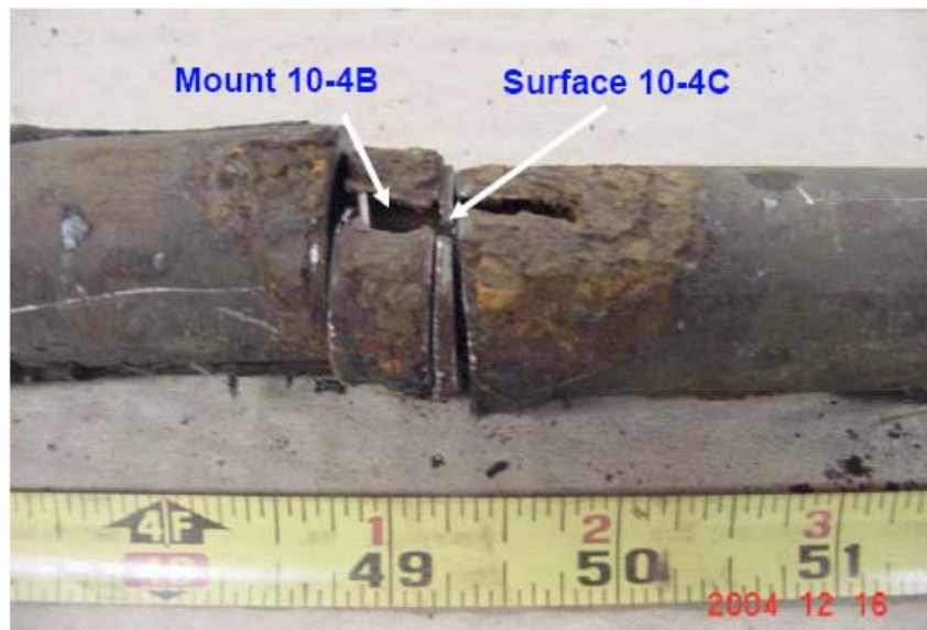
Figure 19. Segment 10 showing Mount 10-4B (2 nd piece from left) and Surface 10-4C (3 rd piece from left).
