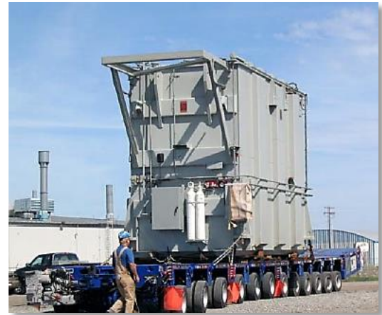
This is one of the largest transformers we purchase. It connects the 230 kV and 115 kV systems.
