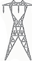
Transmission Nominal Voltage: 500 kV Type: Tower Typical Tower Height: 90-150 feet Typical Right-of-Way Width: 160-200 feet
