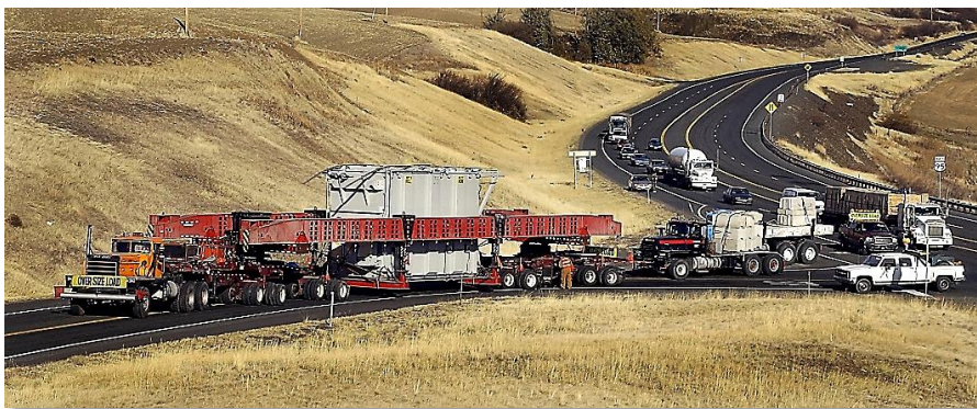
Dry Creek 230/115 transmission auto transformer making its way to Dry Creek Substation
