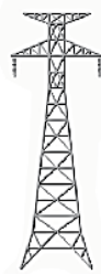
Transmission Nominal Voltage: +/- 400 kV HVDC Type: Tower Typical Tower Height: 145-180 feet Typical Right-of-Way Width: 160-180 feet
