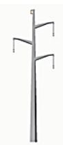
Transmission Nominal Voltage: 161 kV Type: Single Pole Typical Tower Height: 70-95 feet Typical Right-of-Way Width: 100-150 feet
