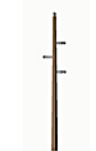
Transmission Nominal Voltage: 69 kV Type: Single Pole Typical Tower Height: 50-70 feet Typical Right-of-Way Width: 70-100 feet
