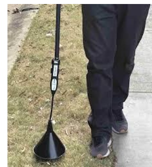
Pipeline Leak Detection
