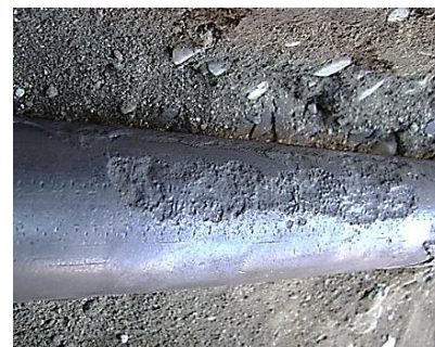
Steel Pipe Corrosion Damage
