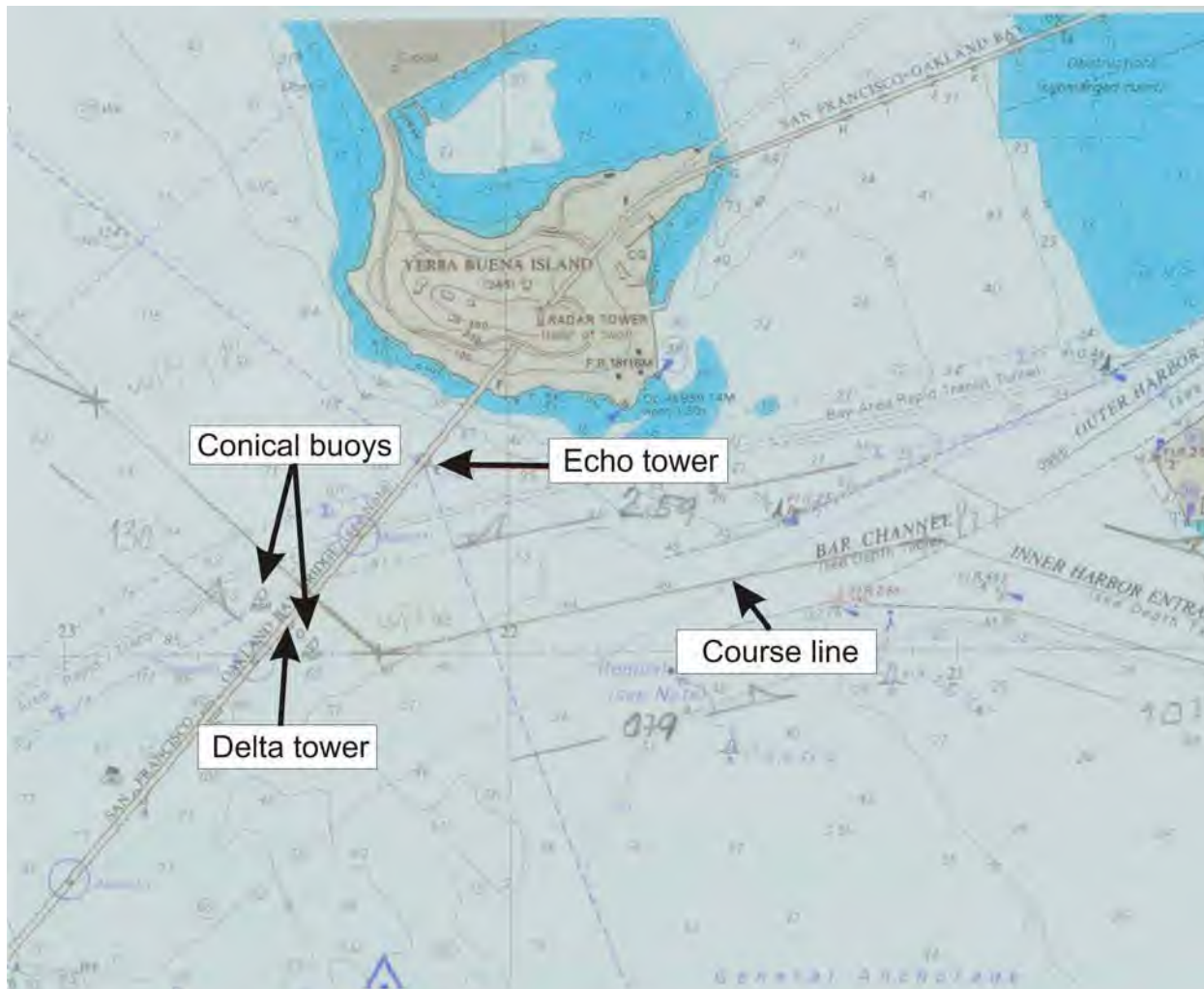
Figure 10. A portion of the paper chart that was on the chart table on the bridge of the Cosco Busan at the time of the allision. The course line, with in- and outbound headings, had been plotted and added to the chart by the ship's crew.
