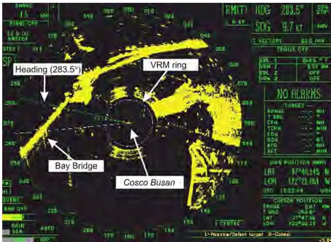
Figure 13. (Top) Radar image displayed on the bridge of the Cosco Busan at 0822:44, just before the vessel turned to port, and (bottom) the radar image at 0826:14, just after the vessel made the turn to port. In the bottom image, note the identifier for the RACON at the center of the Delta–Echo span of the bridge.
