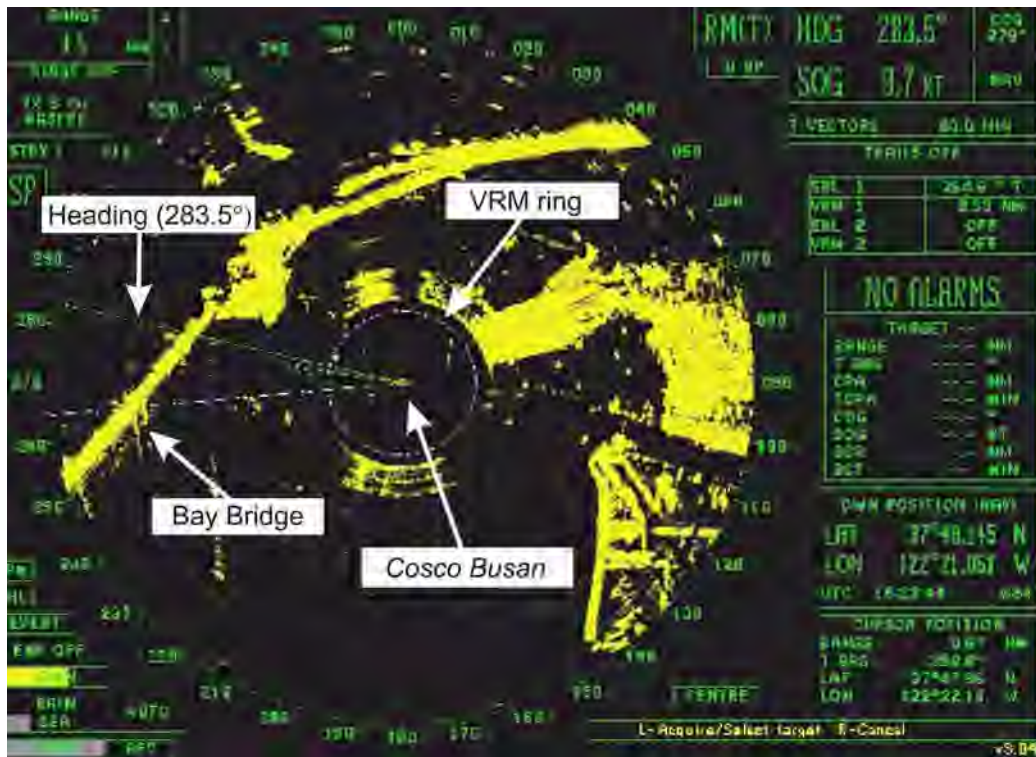
Figure 13. (Top) Radar image displayed on the bridge of the Cosco Busan at 0822:44, just before the vessel turned to port, and (bottom) the radar image at 0826:14, just after the vessel made the turn to port. In the bottom image, note the identifier for the RACON at the center of the Delta–Echo span of the bridge.
