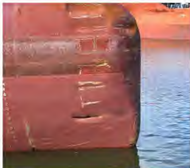
Yochow's bow showing, at left, holed bulbous bow and depth of penetration and, at right, damaged upper starboard bow.
