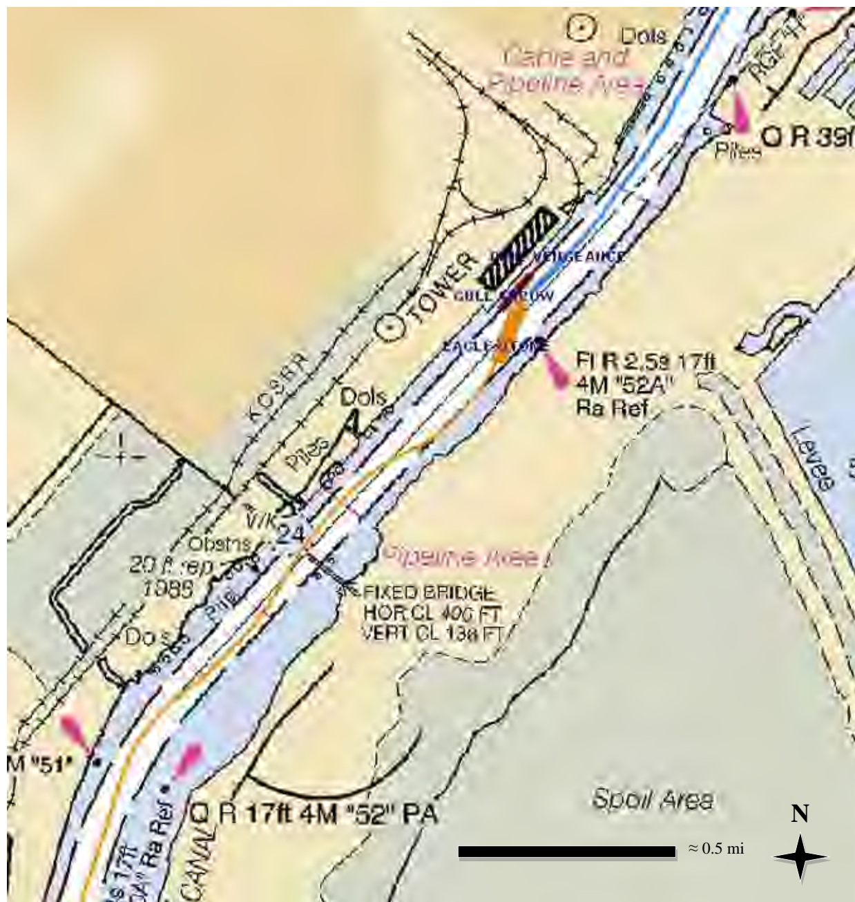
Figure 7. Trackline of the Eagle Otome , obtained from the tankship's S-VDR, overlaid as an orange line on NOAA chart 11342, and trackline of the Dixie Vengeance , obtained from automatic identification system (AIS) 21 data, overlaid as a blue line.
