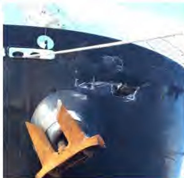
Yochow's bow showing, at left, holed bulbous bow and depth of penetration and, at right, damaged upper starboard bow.
