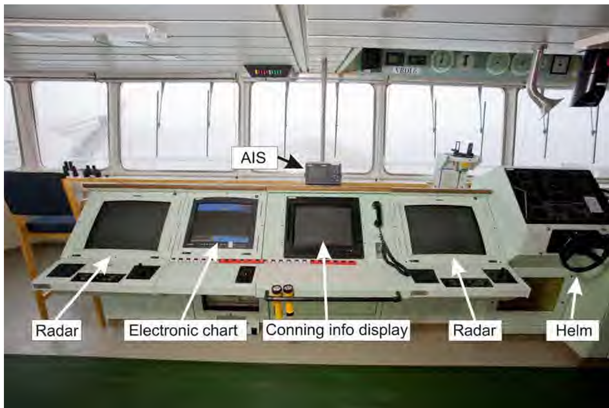
Figure 7. The bridge of the Cosco Busan showing primary navigation displays.
