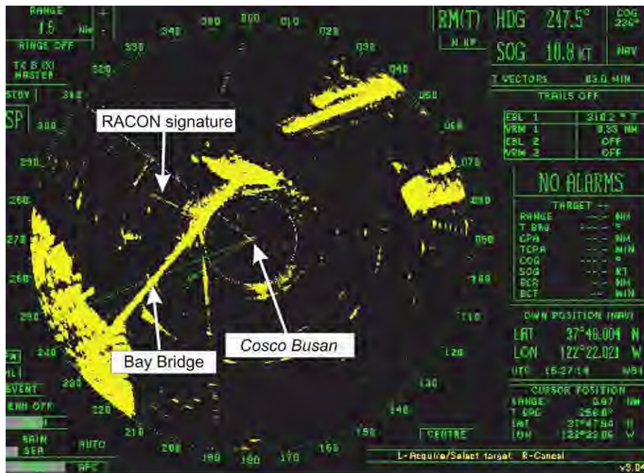
Figure 14. Radar image on board the Cosco Busan at 0827:14. According to investigators, 0827:14 was the time at which the upper portion of the bridge appeared the most enlarged on the radar image before returning to normal.
