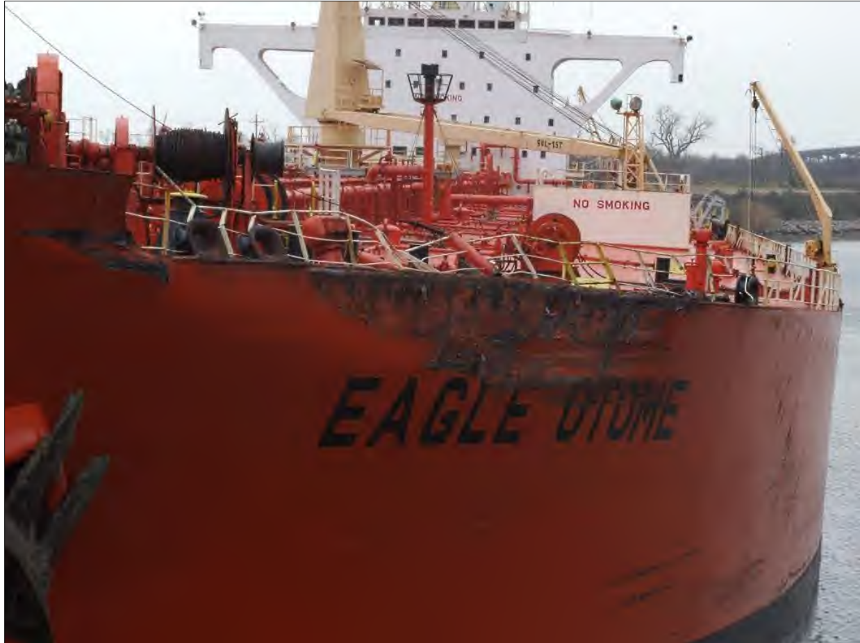
Figure 10. Portside damage to the Eagle Otome .
