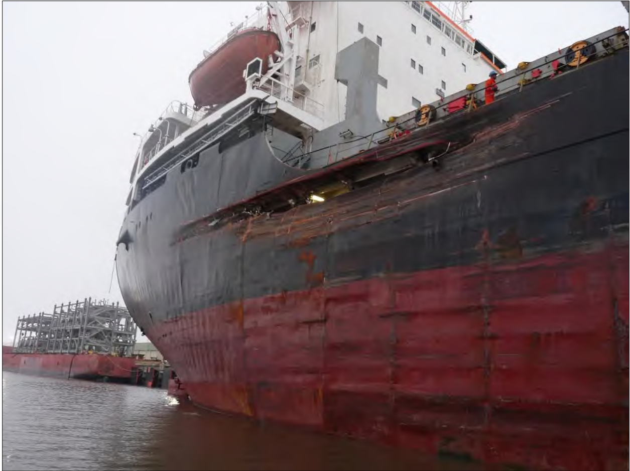
Figure 12. Damage to the Gull Arrow .
