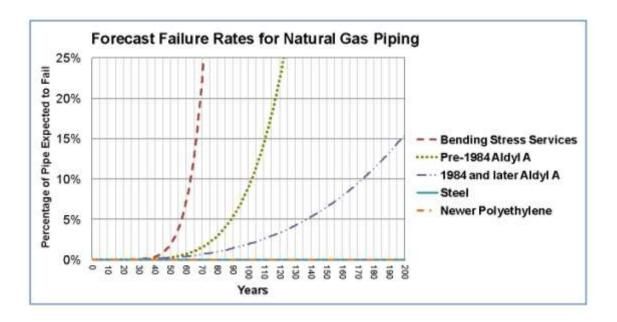
The failure curves show dramatic differences in the expected life for the pipe classes evaluated. The difference in expected life between the Aldyl A products as a group, compared with that of steel and newer-generation plastic pipe, is particularly evident. Striking also, are the expected performance differences among the classes of Aldyl A pipe evaluated, providing some clear trends useful in designing remediation strategies.
