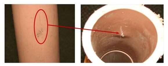
Although the duration of the stress caused by rock contact with the pipe is very different from that associated with squeeze-off, they both result in the same pattern of crack initiation and slow crack growth leading to failure of the pipe. Other sources of external stress that can result in brittle failure of Aldyl A pipe, as mentioned earlier in the report, include bending of the pipe, soil settlement, dents or gouges to the pipe, and improper installation of fittings.
