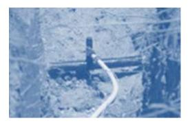
It is at this transition point, between the rigid steel fitting and the more-flexible Aldyl A service pipe, that brittle-like cracking has been observed. This failure mode in older plastic pipe is well understood, and was one of the three study objectives reported by the National Transportation Safety Board in its 1998 bulletin, summarized earlier in this report.
