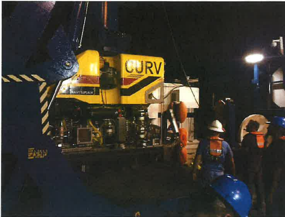
Figure C-4. CURV-21 landing on Apache deck after retrieving VDR.
