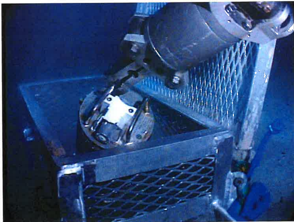
Figure C-3. CURV-21 placing VDR capsule in basket for transport to surface. (US Navy photo)
