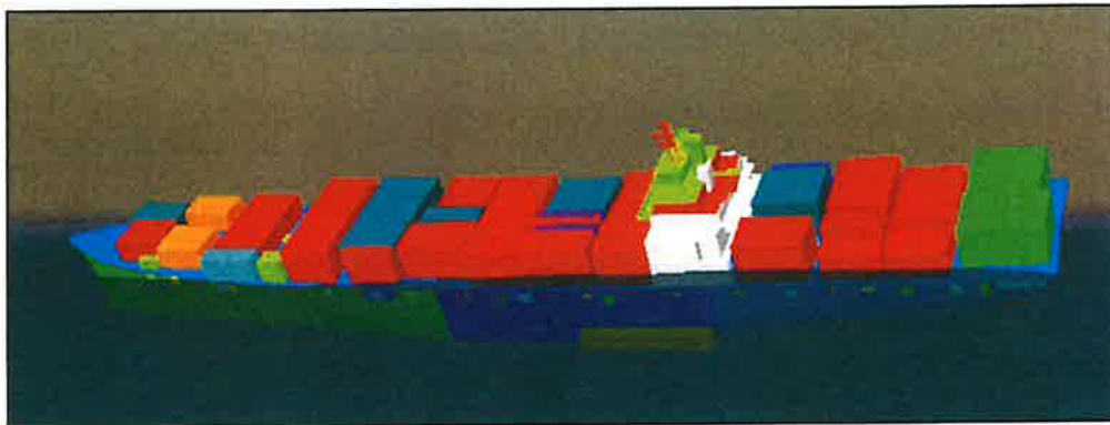
Figure 61. El Faro rolling about a 15° to 18° static heel with waves or green water reaching ventilation openings after propulsion loss. (Screen shot at extreme position from CSRA video simulation)
