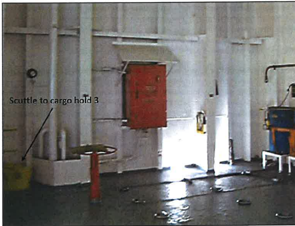
Figure 57. Second deck scuttle to hold 3. (Photo by former El Faro second mate)
