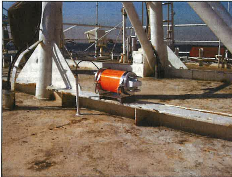
Figure 15. VDR capsule on deck above El Faro 's navigation bridge. (Radio Holland photo 80 )
