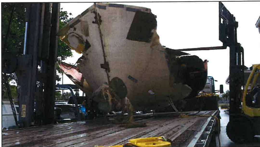
Figure 53. El Faro's starboard lifeboat on arrival at Coast Guard Air Station Miami. Note fouled propeller, bent propeller blade, and damage to port and starboard sides of hull.
